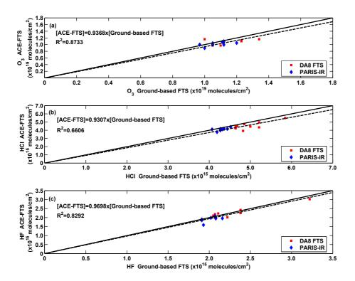
**Fig. 6.** Scatter plot of partial columns measured by ACE-FTS versus those observed by ground-based FTSs for **(a)**  $O_3$ , **(b)** HCl, and **(c)** HF. In all figures, the dotted line shows the fitted correlation function between the two data sets being compared. Results from both the DA8 FTS and PARIS-IR were fit together to in this calculation. The slope and  $R^2$  for the comparisons are given on the figure. The solid line shows the one-to-one relationship for the comparison.
