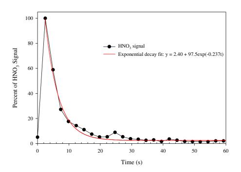
**Fig. 4.** Spike test of the inlet using a  $68 \text{ wt } \% \text{ HNO}_3$  solution exposed to the 12 ft inlet for less than one second. The data was collected at 0.4 Hz.
