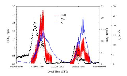
**Fig. 8.** Gaseous HNO<sub>3</sub>, aerosol nitrate (NO<sub>3</sub>), and the calculated dissociation constant  $K_{\rho}$  of Reaction 18 for 22 and 23 March 2006.
