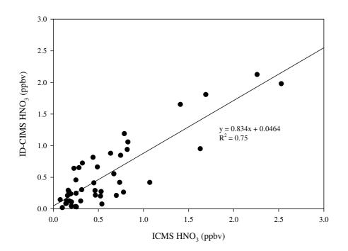
**Fig. 10.** Inter-comparison between the ID-CIMS and ICMS based on 45 overlapping data points collected from 8 to 29 March 2006.
