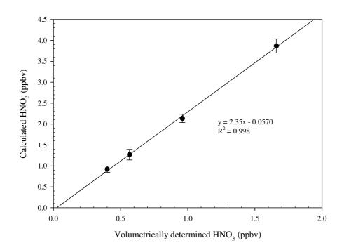
Fig. 2. Plot of calculated verse volumetrically prepared  $HNO_3$  concentrations. The slope corresponds to the calibration factor.
