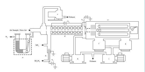
**Fig. 1.** Schematic diagraph of the ID-CIMS: **(a)**, HNO<sub>3</sub> permeation device; **(b)**, ion source; **(c)**, dry scroll pump for air sampling; **(d)**, 10-ring drift tube; **(e)**, Extrel 150-QS mass spectrometer; **(f)** and **(g)**, Varian TV-551 turbo pumps; **(h)**, Edwards E2M30 oil pump; **(i)**, Varian DS402 oil pump.
