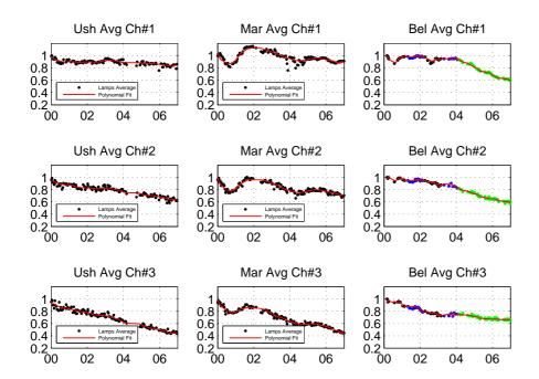
**Fig. 1.** Lamp measurements time series of Ushuaia, Marambio and Belgrano during 2000–2006. Results of the six channels are shown together with the average of the lamps and the polynomial fit. The colors in Belgrano series indicate the different instrumetrs used.
