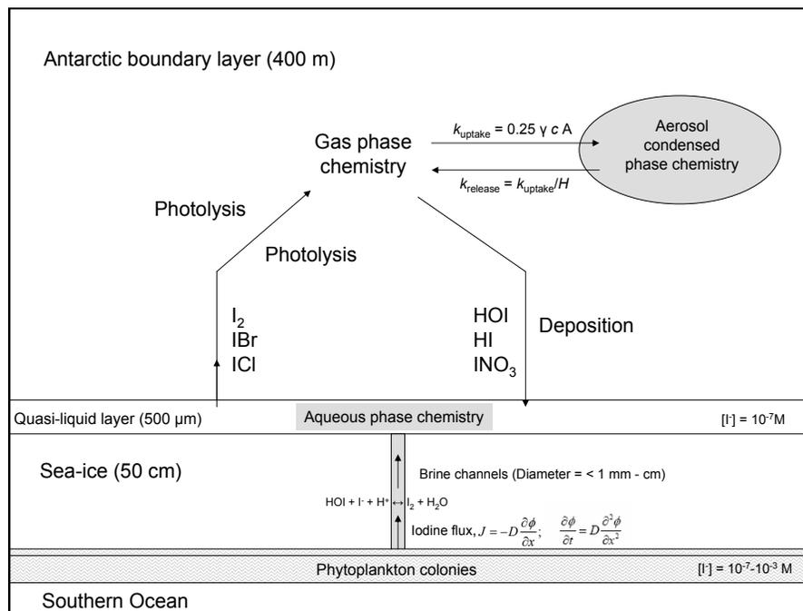
**Fig. 2.** A simplified quantitative schematic of the proposed mechanism and the CON-AIR model structure. Note that the dimensions are not at real scale.
