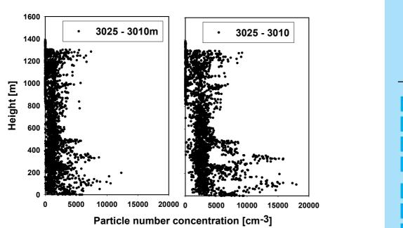
Fig. 7. (Left) Aerosol concentration for sizes 3 nm<D<6 nm and (Right) 6 nm <D<10 nm.
