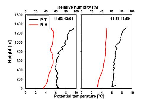
Fig. 5. Potential temperature and relative humidity boundary layer structure for 25 March 2003.
