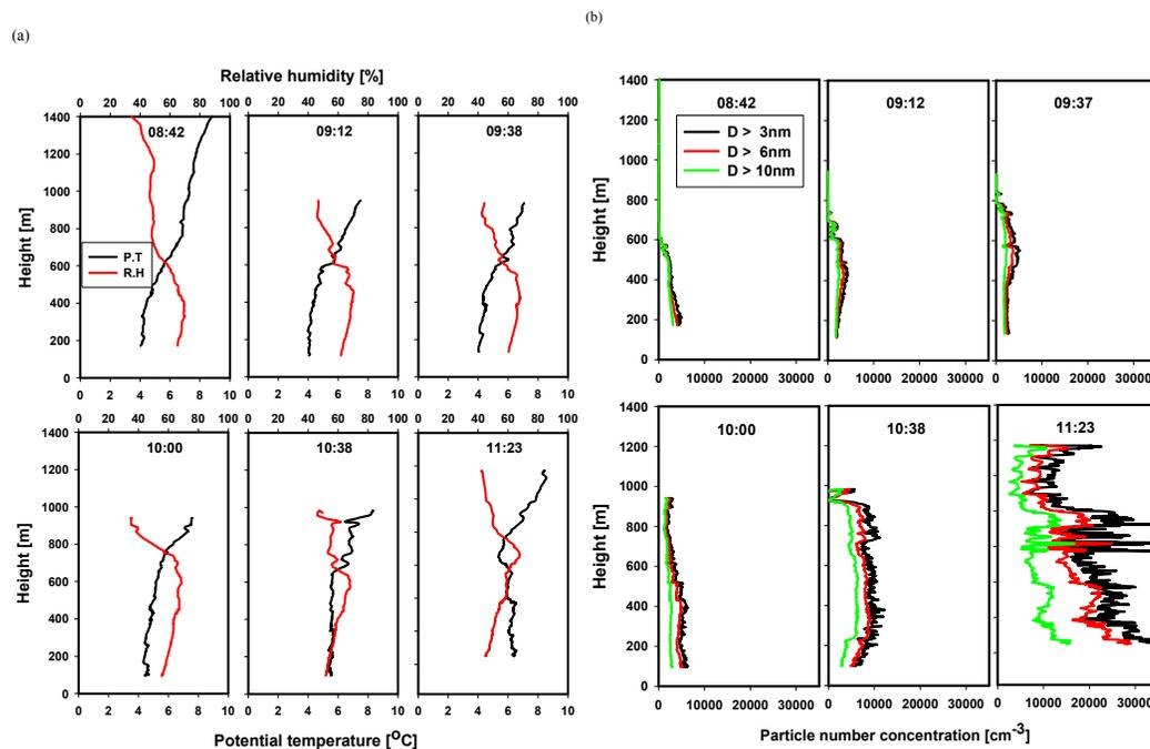
**Fig. 12.** (a) evolution of boundary layer structure, as determined by potential temperature and relative humidity, for 28 March 2003. (b) variation in aerosol vertical structure throughout the morning of 28 March 2003. Local time is also listed in each plot.
