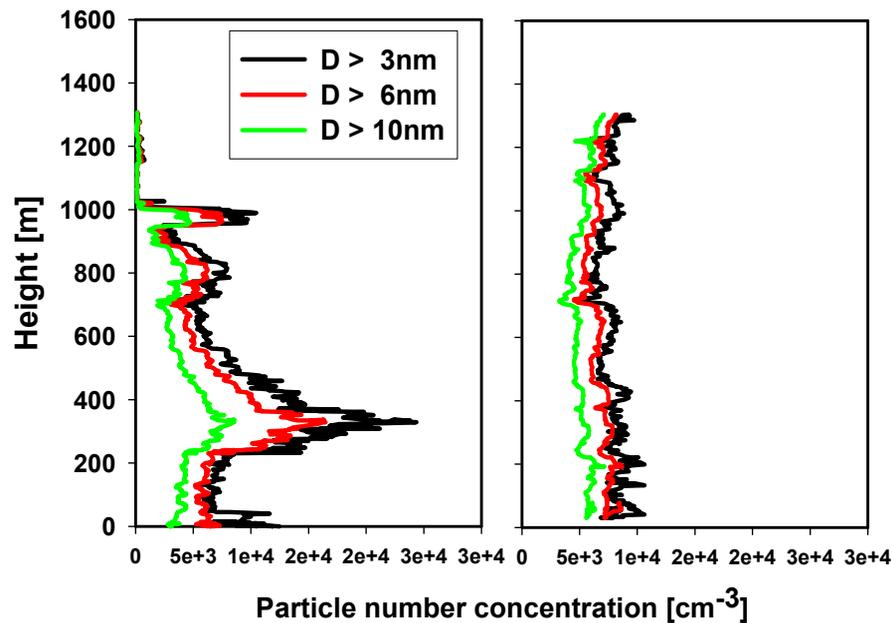
**Fig. 6.** Aerosol boundary layer structure for 25 March 2003. Total number concentration for sizes  $D > 3$  nm, 6 nm and 10 nm.
