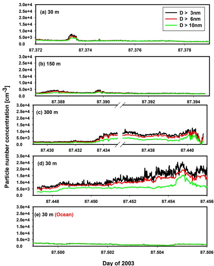
**Fig. 13.** Particle concentration at sizes  $D > 3$ , 6, and 10 nm for horizontal runs at 30, 150 and 300 m over the forest canopy. Also shown is the particle concentration for a 30 m horizontal run over the sea.
