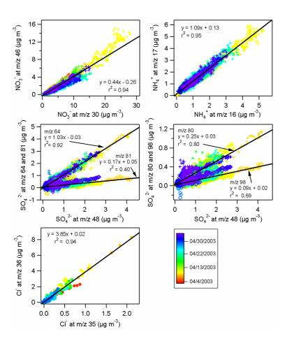
**Fig. 2.** Correlations between the time series of the main fragments used to calculate mass concentration of the inorganic species for the CENICA AMS. Black lines are linear fits to the data.
