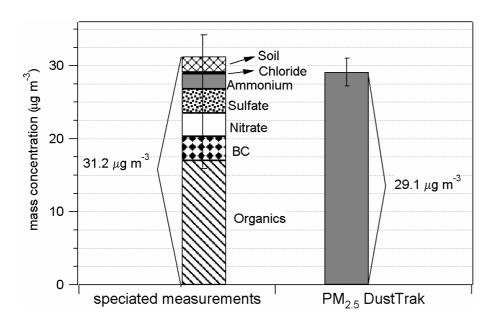
**Fig. 10.** Estimation of the total PM<sub>2.5</sub> mass concentration from AMS, BC, and soil mass concentration, compared with PM<sub>2.5</sub> DustTrak mass concentration. Averages were carried out over all time intervals for which all data (AMS, BC, soil, and DustTrak) were available.
