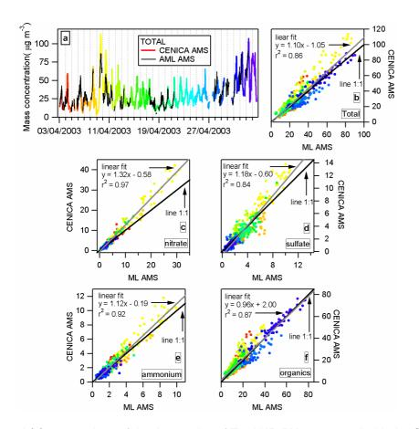
**Fig. 6.** Panel **(a)**: comparison of the time series of Total NR-PM<sub>1</sub> measured with the CENICA and the mobile laboratory AMSs, for periods when the AML was parked at CENICA during MCMA-2003. Panels **(b)** though **(f)**: scatter plots of the Total NR-PM<sub>1</sub>, and its species, measured with the CENICA and the mobile laboratory AMSs. Black lines are 1:1 lines. Grey lines are linear fits to the data. The data is presented in 30 min averages.
