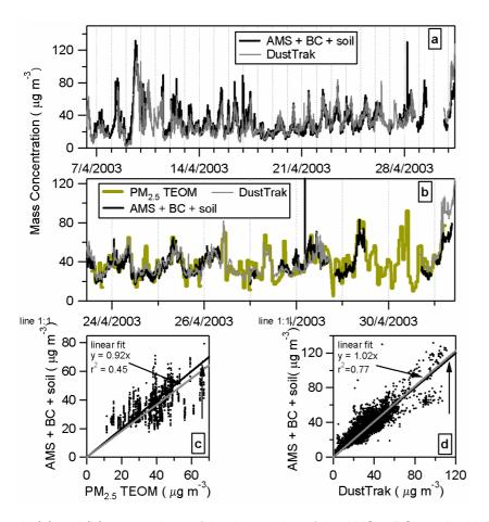
**Fig. 7.** Panels **(a)** and **(b)**: comparison of the time series of the AMS + BC + soil with DustTrak and TEOM PM<sub>2.5</sub> mass concentrations. Panels **(c)** and **(d)**: scatter plots and linear fits for the above comparisons. Grey lines are linear fits to the data.
