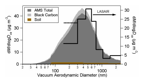
**Fig. 8.** Comparison of the (AMS + estimated BC + soil) and LASAIR size distributions. The BC, AMS and soil size distributions are stacked. The dashed line represents the mass concentration of the smallest LASAIR size channel multiplied by two in order to account for the 50% collection efficiency in this channel.
