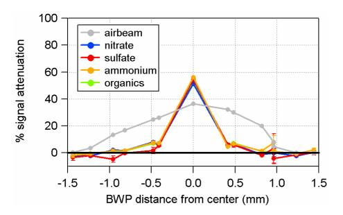
**Fig. 3.** Campaign-average signal attenuation for the airbeam and the main CENICA AMS species as a function of distance of the BWP from the center of the vaporizer. Nitrate, sulfate, and organics curves are not visible because they are behind the ammonium curve.
