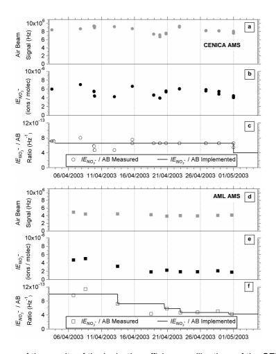
**Fig. 1.** Summary of the results of the ionization efficiency calibrations of the CENICA (panels **a–c**) and Mobile Laboratory (panels **d–f**) AMSs during the MCMA-2003 field campaign.
