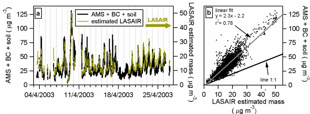
**Fig. 9.** Panel (a): Comparison of the time series of the AMS + BC + soil mass concentration and the estimated mass concentration from the LASAIR instrument. Panel (b): scatter plot and linear fit between both measurements. The grey line is a linear fit to the data.
