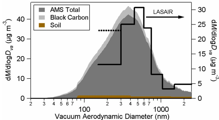
**Fig. 8.** Comparison of the (AMS + estimated BC + soil) and LASAIR size distributions. The BC, AMS and soil size distributions are stacked. The dashed line represents the mass concentration of the smallest LASAIR size channel multiplied by two in order to account for the 50% collection efficiency in this channel.
