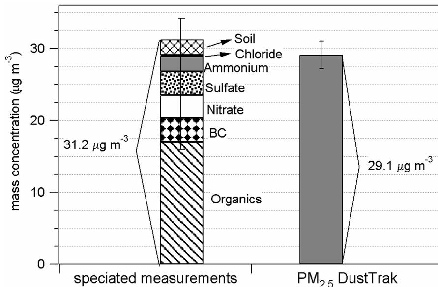
**Fig. 10.** Estimation of the total PM<sub>2.5</sub> mass concentration from AMS, BC, and soil mass concentration, compared with PM<sub>2.5</sub> DustTrak mass concentration. Averages were carried out over all time intervals for which all data (AMS, BC, soil, and DustTrak) were available.
