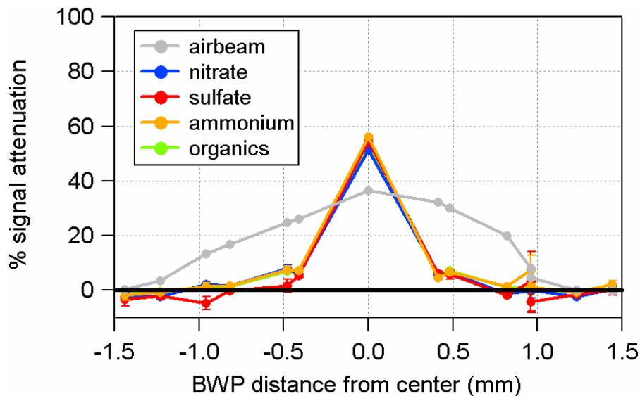
**Fig. 3.** Campaign-average signal attenuation for the airbeam and the main CENICA AMS species as a function of distance of the BWP from the center of the vaporizer. Nitrate, sulfate, and organics curves are not visible because they are behind the ammonium curve.
