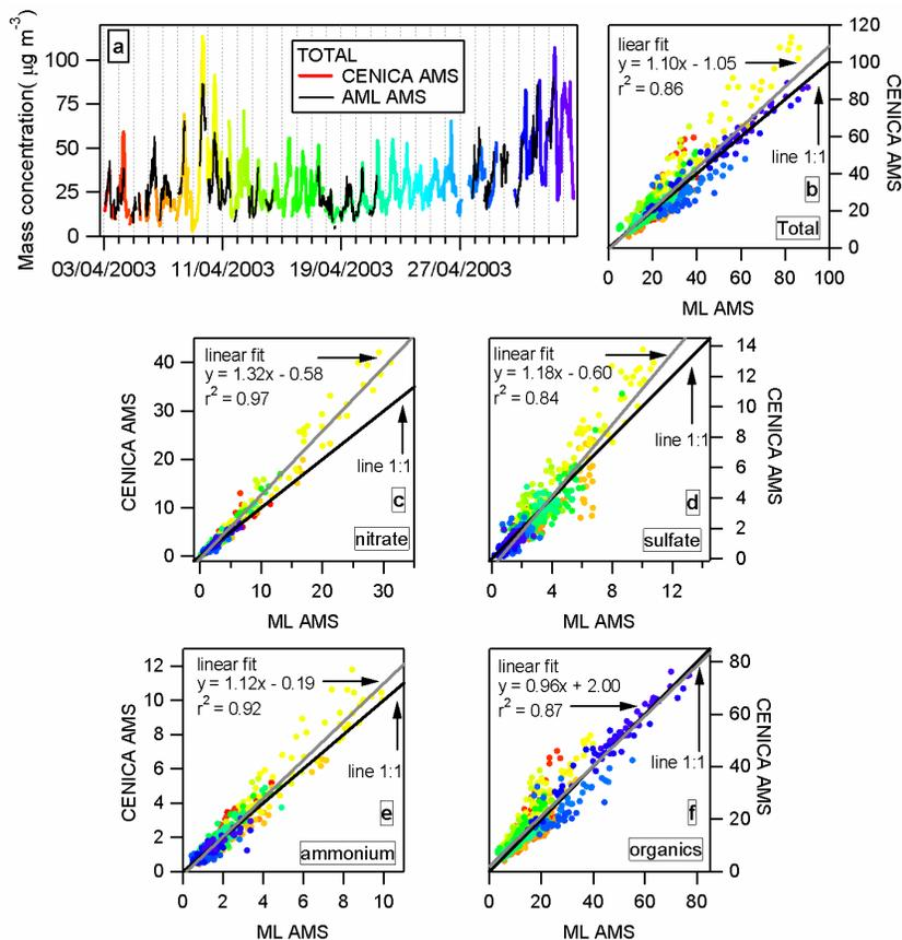
**Fig. 6.** Panel (a): comparison of the time series of Total NR-PM<sub>1</sub> measured with the CENICA and the mobile laboratory AMSs, for periods when the AML was parked at CENICA during MCMA-2003. Panels (b) through (f): scatter plots of the Total NR-PM<sub>1</sub>, and its species, measured with the CENICA and the mobile laboratory AMSs. Black lines are 1:1 lines. Grey lines are linear fits to the data. The data is presented in 30 min averages.
