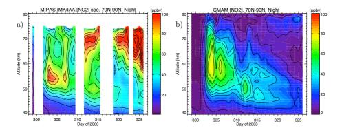
**Fig. 6.** Time series of NO<sub>2</sub> enhancement after the solar proton events of October–November 2003 for the Northern Hemisphere polar cap (70–90° N) at nighttime conditions as measured by MIPAS **(a)** and modeled by the Canadian Middle Atmosphere Model (CMAM) **(b)**. The vertical white bands in panel (a) represent days with no processed data.
