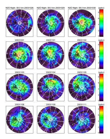
**Fig. 1.** Northern Hemisphere distributions of  $N_2O$  (in ppbv, parts per billion by volume) for days from 26 October to 11 November 2003 at an altitude of 58 km. Only nighttime data is included. Contours are zonally smoothed within 700 km. Individual measurements are represented by white symbols.
