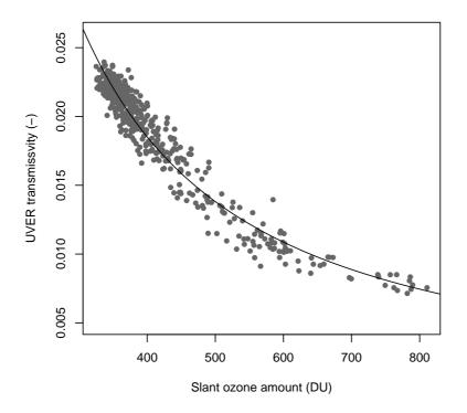
**Fig. 4.** Power law regression between UVER atmospheric transmissivities and slant ozone amount for clear cases at Badajoz from February 2001–December 2005. The coefficient of the power law function (1.31) gives the RAF value.
