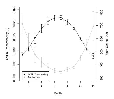
**Fig. 3.** The monthly mean evolution of slant ozone column and UVER transmisivity (only cloud-free conditions) at Badajoz station.
