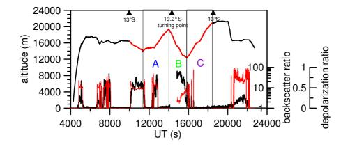
**Fig. 2.** Time series of the altitude profile of the Geophysica flight (black line, vertical axis on the left) and backscatter and aerosol depolarization ratio from the backscattersonde (black and red lines respectively, vertical axis on the right). Triangles denote geographical locations of interest. Three portions of the flight, indicated here as A, B, and C sections, are used to derive atmospheric vertical profiles in the following figures.
