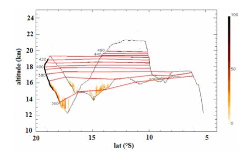
**Fig. 3.** Colour coded backscatter ratio along the flight path from the backscattersonde MAS, and above it from the miniaturized lidar MAL, function of latitude and height. Black line is the aircraft flight path. The thicker black line denotes a loss of MAS data at the southernmost edge of the flight. Red lines connects points of equal potential temperature (as tagged) along the flight path.
