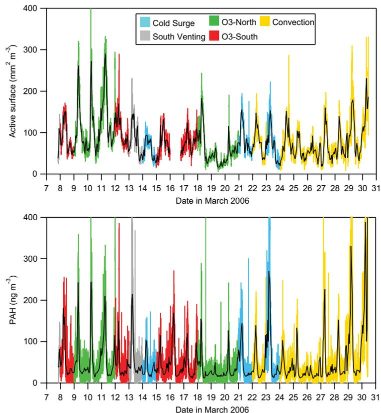
**Fig. 2.** AS and PAH concentrations at T0 during the entire field campaign. Raw 1-min measurements are shown by the colored lines, where color indicates the wind transport episode, and 1-h averages are shown in black.
