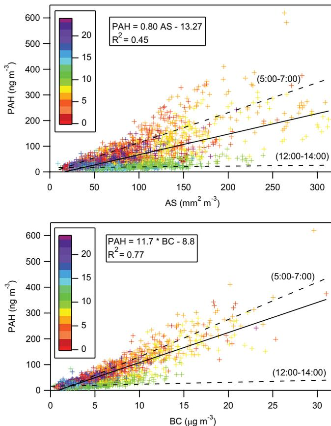
**Fig. 4.** PAH v. AS and PAH v. BC concentrations at T0 colored by hour. The solid line is the linear regression for all times, and its equation is shown in the box. The dotted lines labeled 05:00–07:00 and 12:00–14:00 are the regressions for a subset of data specific to these time periods. The equations of these lines are given in the text.
