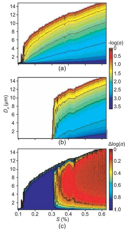
**Fig. 3.** (a)  $\alpha(S, D)$  for 30 s of droplet growth on ammonium sulfate particles (100% soluble) with  $D_{\text{dry}}=100$  nm. (b) Same as (a), but with 5% soluble particles. (c) Difference between (a) and (b).
