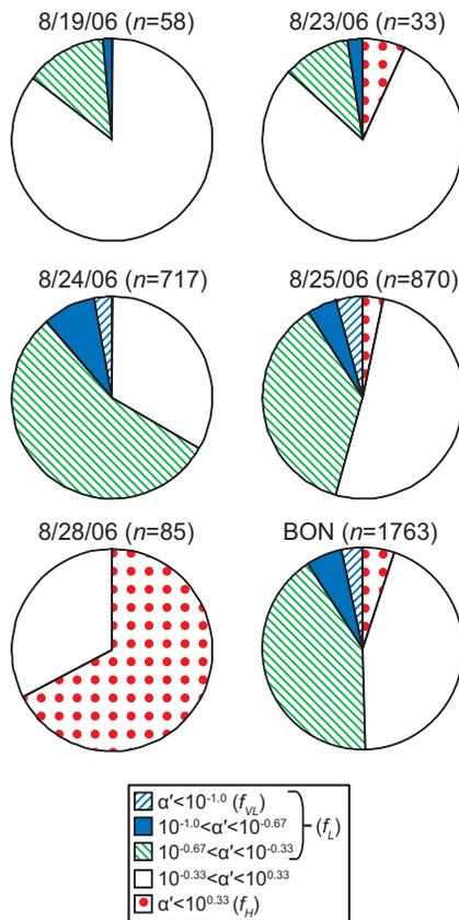
**Fig. 7.** Summary of CCN  $\alpha'$  distributions for each day at BON, and the total from the site. An  $\alpha'$  of  $10^{-1.0}$  is  $6\sigma$  below the mean for ammonium sulfate ( $\alpha_{app,AS}$ ),  $\alpha' = 10^{-0.67}$  is  $4\sigma$  below  $\alpha_{app,AS}$ ,  $\alpha' = 10^{-0.33}$  is  $2\sigma$  below  $\alpha_{app,AS}$ , and  $\alpha' = 10^{0.33}$  is  $2\sigma$  above  $\alpha_{app,AS}$ .
