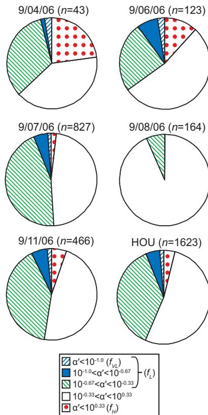
**Fig. 8.** Summary of CCN  $\alpha'$  distributions for each day at HOU, and the total from the site. An  $\alpha'$  of  $10^{-1.0}$  is  $6\sigma$  below the mean for ammonium sulfate ( $\alpha_{app,AS}$ ),  $\alpha' = 10^{-0.67}$  is  $4\sigma$  below  $\alpha_{app,AS}$ ,  $\alpha' = 10^{-0.33}$  is  $2\sigma$  below  $\alpha_{app,AS}$ , and  $\alpha' = 10^{0.33}$  is  $2\sigma$  above  $\alpha_{app,AS}$ .
