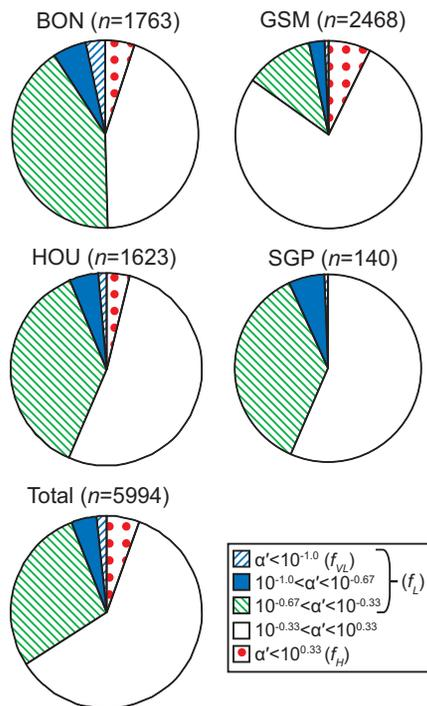
**Fig. 5.** Summary of CCN  $\alpha'$  distributions at each site, and the total of all four sites. An  $\alpha'$  of  $10^{-1.0}$  is  $6\sigma$  below the mean for ammonium sulfate ( $\alpha_{app,AS}$ ),  $\alpha'=10^{-0.67}$  is  $4\sigma$  below  $\alpha_{app,AS}$ ,  $\alpha'=10^{-0.33}$  is  $2\sigma$  below  $\alpha_{app,AS}$ , and  $\alpha'=10^{0.33}$  is  $2\sigma$  above  $\alpha_{app,AS}$ .
