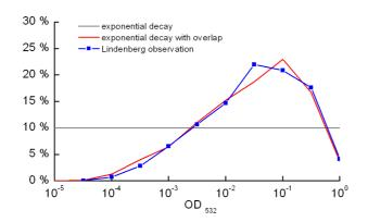
**Fig. 1.** Frequency of occurrence of optical depths measured with the MARL lidar in Lindenberg from May 2003 to October 2003 (blue line). The red and grey lines show simulated curves based on an exponential decay of clouds with time allowing and not allowing for temporal overlap of clouds, respectively.
