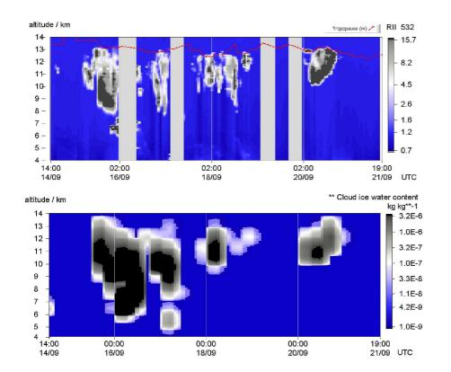
**Fig. 6.** The upper plot shows lidar observations of cirrus clouds in term of the backscatter ratio at 532 nm for one week in September 2003. The lower plot shows the corresponding cloud ice water content at the nearest gridpoint to Lindenberg (52°, 14°) of opECMWF for the same time period.
