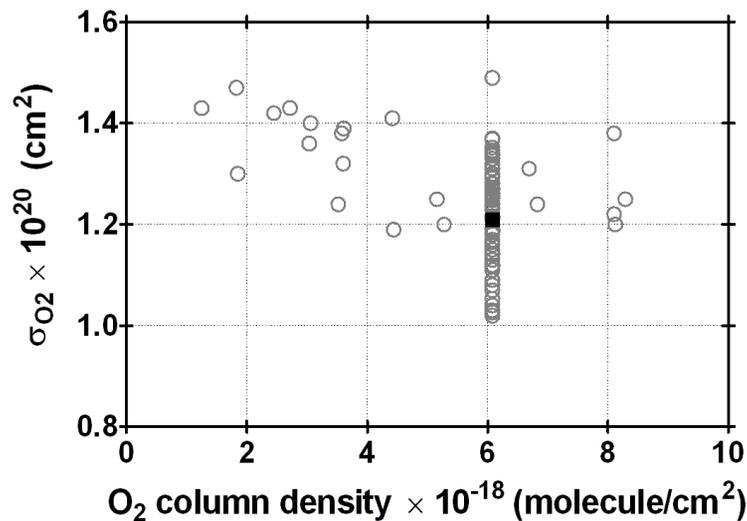
**Fig. 3.** Oxygen absorption cross-sections measured as a function of  $O_2$  column density. The grey circles are individual measurements performed at various conditions of lamp temperatures and voltages. The dark square is an average of 101 measurements performed at a typical  $O_2$  column density of  $6.1 \times 10^{-18}$  molecule/cm<sup>2</sup> used during OH calibrations. The average leads to  $\sigma_{O_2} = 1.21 \times 10^{-20}$  cm<sup>2</sup> with a standard deviation of 0.8%.
