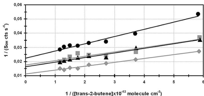
**Fig. 8.** Plot of  $1/S_{OH}$  versus  $1/[\text{trans-2-butene}]$  for 4 independent calibrations at various  $[\text{O}_3]$ ,  $[\text{water}]$  and laser power: ●2.1 ppm  $\text{O}_3$ , 0.75% water, 1.0 mW; ■2.2 ppm  $\text{O}_3$ , 0.47% water, 1.0 mW; ▲2.5 ppm  $\text{O}_3$ , 0% water, 0.9 mW; ◇2.4 ppm  $\text{O}_3$ , 0% water, 1.4 mW.
