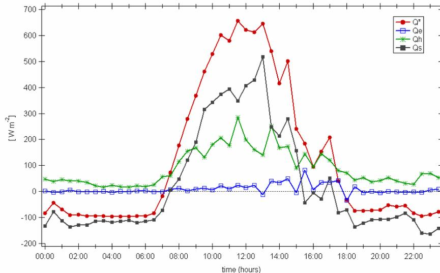
**Fig. 3.** Energy balance measured on 24 March 2006 in the urban core of Mexico City during the MILAGRO field campaign. The sensible ( $Q_h$ ) and latent ( $Q_e$ ) heats were measured by eddy covariance,  $Q^*$  by a net radiometer and  $\Delta Q_s$  was obtained as the residual of the measured energy components ( $\Delta Q_s = Q^* - (Q_h + Q_e)$ ) (Velasco et al., 2007<sup>1</sup>).
