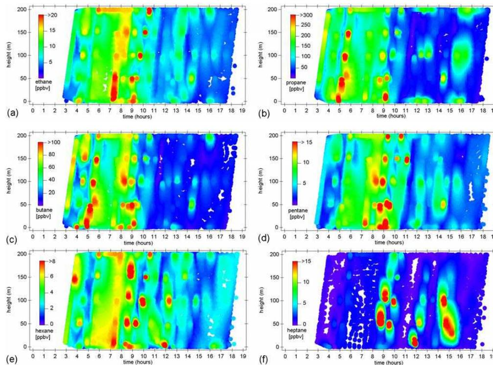
**Fig. 6.** Vertical distributions of the 13 VOCs monitored. **(a)** ethane, **(b)** propane, **(c)** butane, **(d)** pentane, **(e)** hexane, **(f)** heptane, **(g)** octane, **(h)** nonane, **(i)** propylene, **(j)** acetylene, **(k)** benzene, **(l)** toluene, **(m)** o-xylene.
