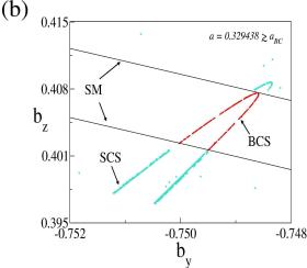
**Fig. 8.** Transition from a chaotic attractor to a chaotic saddle via a boundary crisis (BC). (a) Post-BC surrounding chaotic saddle (SCS, blue) and banded chaotic saddle (BCS, red) at  $a=0.329438 \gtrsim a_{\rm BC}$ ; (b) a zoom of (a), the thin line denotes the stable manifold (SM) of the mediating unstable periodic orbit.
