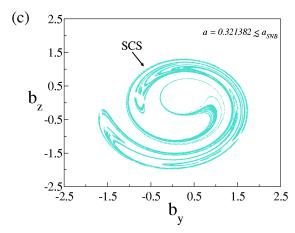
**Fig. 6.** Transition from a chaotic saddle to a chaotic attractor via a saddle-node bifurcation. **(a)** Post-SNB chaotic saddle at  $a_{\rm SNB}$ =0.321383; **(b)** pre-SNB chaotic attractor at a=0.321382 $\lesssim a_{\rm SNB}$ ; **(c)** pre-SNB chaotic saddle embedded in the chaotic attractor at a=0.321382 $\lesssim a_{\rm SNB}$ .
