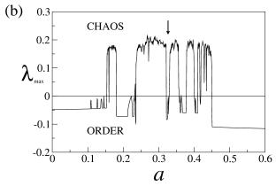
**Fig. 1.** Limit point diagram and maximum Lyapunov exponent: global view. (a) Limit point diagram,  $b_z$  as a function of the driver amplitude a; (b) maximum Lyapunov exponent  $\lambda_{\text{max}}$  as a function of a. The arrow indicates a period-3 periodic window.  $\nu$ =0.02,  $\Omega$ =-1,  $\lambda$ =1/4,  $\mu$ =1/2.
