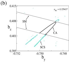
**Fig. 7.** Chaotic attractor-chaotic saddle collision at boundary crisis (BC) for  $a_{\rm BC}$ =0.329437. (a) Pre-BC surrounding chaotic saddle SCS (blue) and banded chaotic attractor CA (black); (b) a zoom of (a). The cross denotes a fixed point of the p-9 mediating unstable periodic orbit (M) and the thin line denotes its stable manifold (SM).
