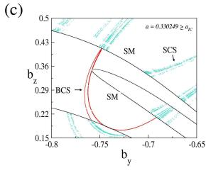
**Fig. 10.** Chaotic attractor and chaotic saddle after the Alfvén interior crisis at a=0.330249 $\gtrsim a_{\rm IC}$ . (a) Poincaré map of the strong chaotic attractor (SCA); (b) the surrounding chaotic saddle (SCS, blue) and the banded chaotic saddle (BCS, red) embedded in the chaotic attractor of (a); (c) enlargement of the rectangular region of (b). SM (thin line) denotes the stable manifold of the mediating unstable periodic orbit of period-9.
