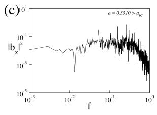
**Fig. 12.** Alfvén crisis-induced intermittency. (a) Time series  $b_z$  as a function of  $\tau$  for a=0.3310, (b) same time series as (a) plotted as a function of driver cycles, (c) power spectrum of (a). SCS denotes surrounding chaotic saddle and BCS denotes banded chaotic saddle.
