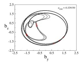
**Fig. 4.** Mediating unstable periodic orbit of period-9 created by a saddle-node bifurcation at  $a_{SNB} = 0.32935$ . The solid line denotes the state-space trajectory, and the cross denotes the Poincaré point.
