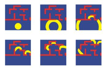
**Fig. 5.** Output of the first layer of a CNN in which a wavefront moves in a 2-D labyrinth. The inputs values of the two layers of the CNN represent the labyrinth (red pixel). The wavefronts of the first layer propagate throughout the medium with a constant speed, breaking into different arms at each fork (yellow pixel).
