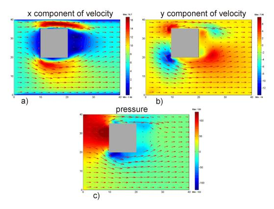
Fig. 8. Distribution of the state variable in a pipeline around an obstacle computed by FEM: surface plot of component of velocity in the (a) x-direction and (b) y-direction, and (c) value of the pressure for an array of  $40 \times 40$  cells. The red arrows are the resultant flux.
