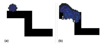
**Fig. 9.** Geometry of the channel used in the simulation using a CNN model as solver of PDE. The value of the state of the system is showed in two different instants of time (a) and (b) of the simulation.
