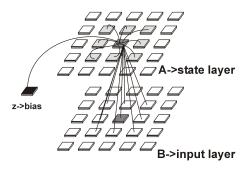
**Fig. 2.** Multilayer CNN (MCNN) composed by cells having several state variables, one for each layer. The interaction between the state variables that belong to different layers can be complete, while the cell-to-cell interaction is restricted to neighbours.
