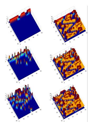
**Fig. 4.** In the left side, it is shown the output of the first layer of the CNN processing a spiral wave with different time constant for each cell. In the right side, capacitor values, used to represent the topography, are overlapped to the output of the first layer of CNN model, opportunely normalized.
