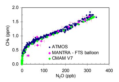
**Fig. 6.** Correlation between  $CH_4$  and  $N_2O$  mixing ratios as measured during the MANTRA campaign of 1998 compared with ATMOS measurements for mid-latitudes and CMAM.
