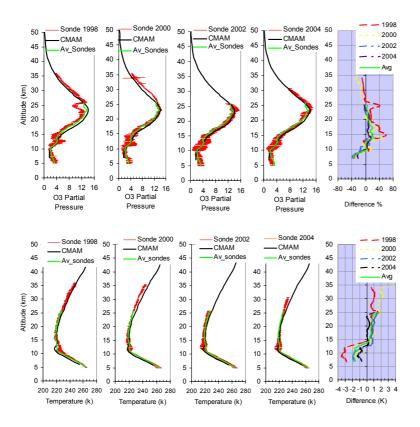
**Fig. 4.** Ozone (upper panels) and temperature (bottom panels) sonde measurements during the four MANTRA campaigns. Also shown is CMAM climatology for August–September covering the measurement period (see text). The differences between each yearly averaged profile (measurement) to the model average for all campaigns (CMAM), for ozone (in percent: ((CMAM-MANTRA)×100/MANTRA) and for temperature (in Kelvin: CMAM-MANTRA), are shown on the right-hand panels, respectively.
