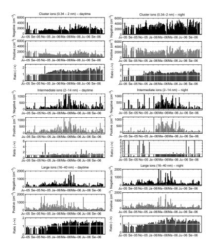
**Fig. 6.** 3-day median ion concentrations (black – negative, grey – positive) and ion ratio (–/+) for cluster (top), intermediate (middle), and large ions (bottom) during July 2005–October 2006. Left column – daytime, right column – nighttime.
