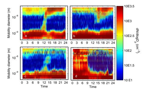
**Fig. 1.** Classification of new-particle formation in Tumbarumba: **(a)** normal, **(b)** Aitken, **(c)** interrupted, and **(d)** nocturnal (see Sect. 2.2 for explanation). At the bottom of each size distribution plot is the band of cluster ions (0.34–1.8 nm). At the top (~25 to 40 nm) is the start of the Aitken mode. Particles between these two modes are called intermediate. Colour indicates the number concentration of particles.
