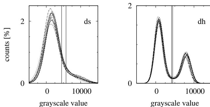
**Fig. 3.** Histograms of the filtered 3-D grayscale tomography images. Shown are all tomograms for decomposing snow and depth hoar. The fraction of “mixed voxels” is much higher for decomposing snow (*ds*) than for depth hoar (*dh*). The bars are located at plus and minus one standard deviation of the mean optimal threshold of the individual measurements.
