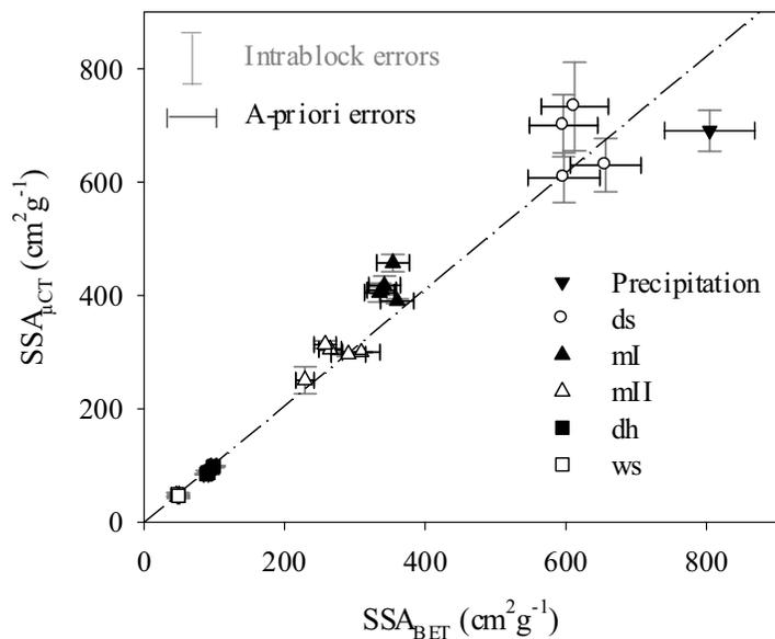
**Fig. 4.** The correlation between adsorption measurements and tomography was found to be  $SSA_{\mu CT} = 1.03(\pm 0.03)SSA_{BET}$ . The plotted error bars given for the adsorption method were called “a-priori errors” whereas the one given for tomography were called “intrablock errors” (see text for details). The data point called “Precipitation” was not taken into account when calculating the correlation coefficient as explained in Sect. 3.3.
