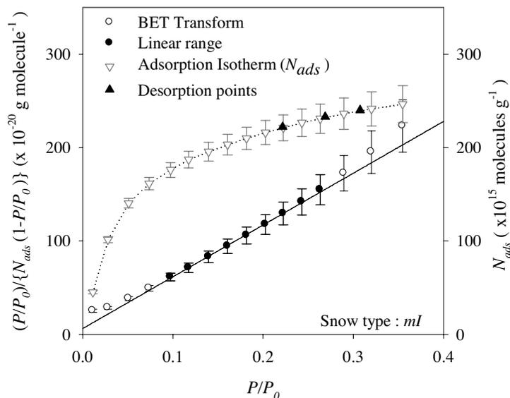
**Fig. 2.** The BET transform (in black on the left axes), is derived from the isotherm of adsorption (in gray on the right axes) (Brunauer et al., 1938). The slope and the intercept of the linear part are used to calculate the SSA (Legagneux et al., 2002).
