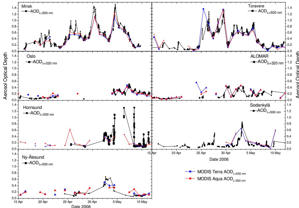
**Fig. 7.** Comparison of  $1^\circ \times 1^\circ$  grid averaged MODIS AOD and AOD from the ground based stations in the period 15 April–15 May 2006. The MODIS AOD from Aqua and Terra is the red and blue curves respectively in all panels.
