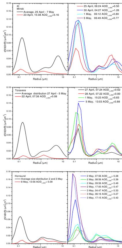
**Fig. 5.** Volume aerosol size distributions during the smoke transport event: **(a)** Minsk, **(b)** Toravere, **(c)** Hornsund. Right panel: Average distribution of the most intense period together with typical distribution. Right panel: Selected distributions during the period. AOD is given at 500 nm.
