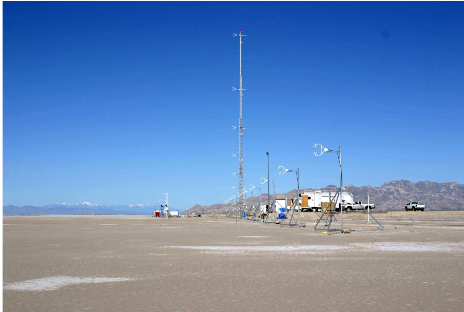
Fig. 1. Looking East at the array of CSAT3 sonic anemometers at the SLTEST site in May, 2005. The instruments were placed forward of a raised causeway (where the vehicle on the right is parked) and berm (where the trailers are parked), giving about 100 km of unobstructed fetch for winds from Northerly directions. Beyond the sonic array, on the playa, is a 5-m tower and two instrument trolleys. These were used in other experiments.
