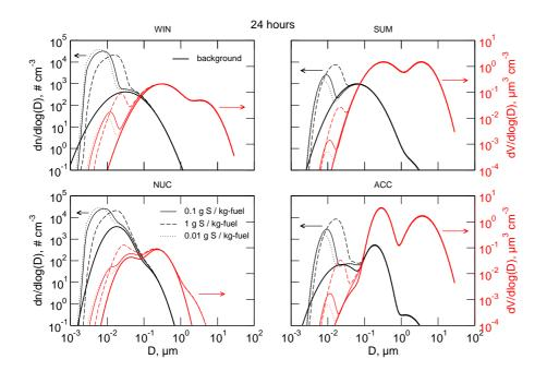
**Fig. 5.** Total number and volume distributions for the four background aerosol cases 24 h after emission for three FSCs. For comparison, the background distributions are shown as thick curves in each panel.
