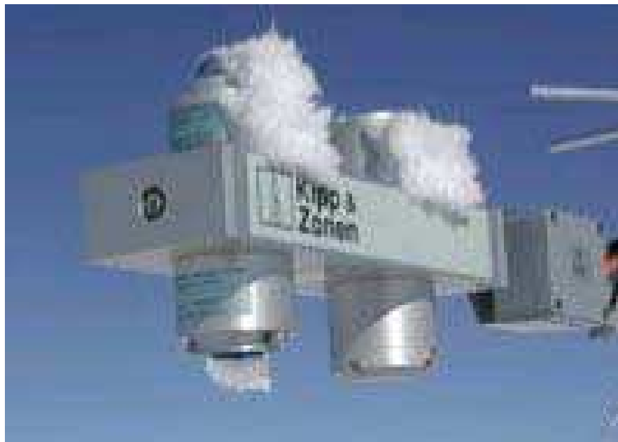
Fig. 11. Four-component radiation sensor on AWS9, at Kohnen Station, Antarctica (CNR1, from Kipp and Zonen). Icing can be a problem on these sensors, but careful cross-analysis of the data can indicate when icing is present. Photo courtesy of M. R. van den Broeke.
