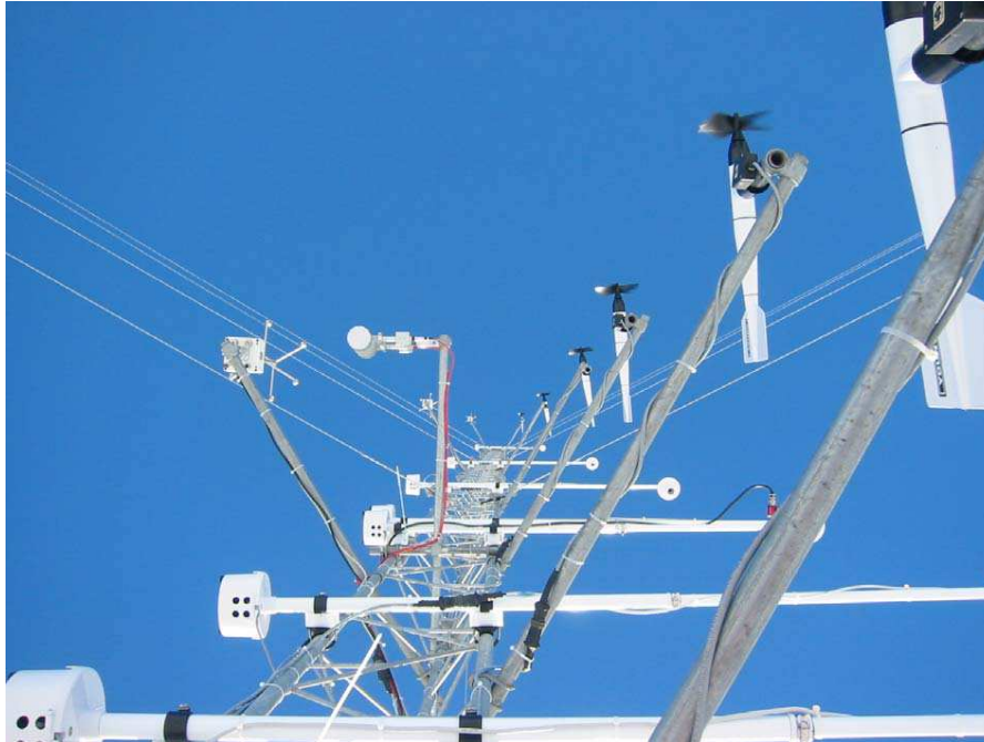
Fig. 12. View up a typical boundary layer profile mast, showing (on RHS) mean wind and temperature sensors at 1, 2, 4, 8, 16 and 32 m levels. On the left are turbulence sensors, with three sonic anemometers at 4, 16 and 32 m, and an infra-red hygrometer (IRH) at 4 m. The IRH allows moisture flux to be estimated using the co-variance of humidity with the pseudo-co-located turbulence data. Image from Halley, 2003.
