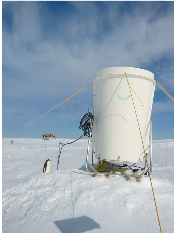
Fig. 13. Simple acoustic sounder (sodar) at Halley. The bulk of the antenna is a hollow cone that acts as acoustic shielding to reduce side echoes and background noise: the base is a focusing dish to produce a vertical acoustic beam for transmission and reception. Off-station acoustic sounders are now available, which use an array of small transceivers to produce the same effect. Note that the antenna is off-vertical due to insolation melting the snow berm.
