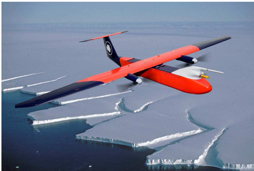
Fig. 14. The Mavionics T200 UAV and Braunschweig University turbulence instrument package being deployed at Halley during 2007 winter. Civilian/research UAVs are developing rapidly, although they are still a high risk instrument platform requiring a skilled operator. Despite GPS waypoint-following robotics able to fly autonomously out of radio/visual contact, at present these units require piloted (radio controlled) take-off and landing. These issues will resolve in time to provide the boundary layer community with an unprecedented view of the spatial structure of the lower atmosphere. Please note that this image is a montage.
