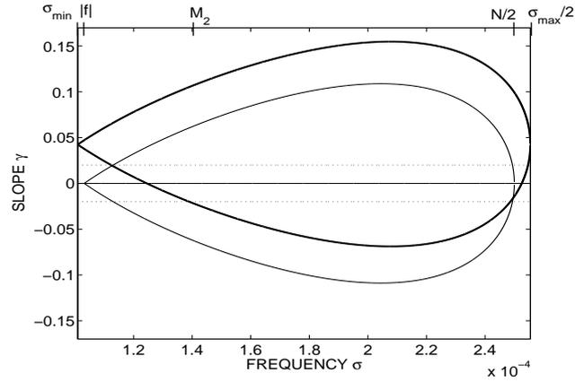
**Fig. 3.** The loci at which the second harmonic is resonantly forced. Thin line: under the Traditional Approximation; thick line: non-traditional. Horizontal dashed lines indicate the range of values covering 67% of the slopes in the ocean. Parameter values are:  $N=5 \times 10^{-4} \text{ rad/s}$  (a value typical of the deep ocean), latitude  $\phi=45^\circ \text{ N}$  and  $\nu=\pi/2$  (propagation in the meridional direction).
