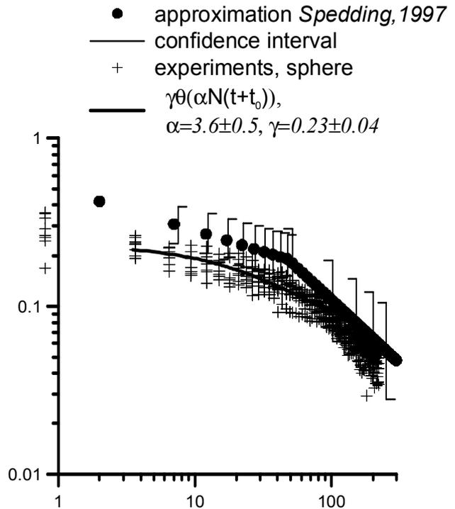
**Fig. 6.** The temporal development of the wake axis velocity according to the experimental data (Spedding, 1997) (crosses), asymptotics  $U_0(t) \sim t^{-0.25}$  and  $U_0(t) \sim t^{-0.76}$  (bullets) and the model prediction (solid curve). Vertical bars show the accuracy of the asymptotics introduced in Spedding (1997).
