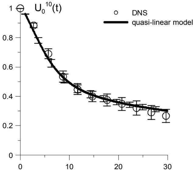
**Fig. 2.** Temporal development of the mean velocity at the axis of the 2-D turbulent jet. Symbols represent the DNS results averaged over 10 different runs. Solid curve corresponds to the model prediction.
