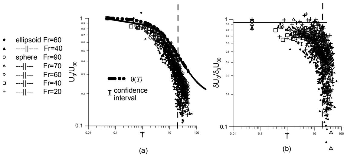
**Fig. 4.** (a) experimental data (symbols) and model solution (solid curve) for the wake axis velocity; the approximation of the velocity by function  $\theta(T)$  (Eq. 13) is shown in dash-dotted curve; (b) temporal development of the product  $U_0(T)\delta(T)$  in the experiment.
