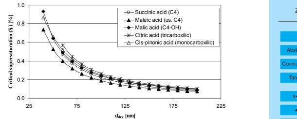
Fig. 5. Critical supersaturation as a function of dry particle diameter for the other organic acids studied.
