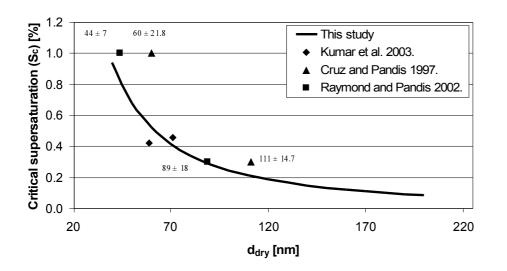
Fig. 7. Comparison of our results for glutaric acid with CCNC data. Data near the points means the confidence interval for results of Cruz and Pandis (1997) and Raymond and Pandis (2002).
