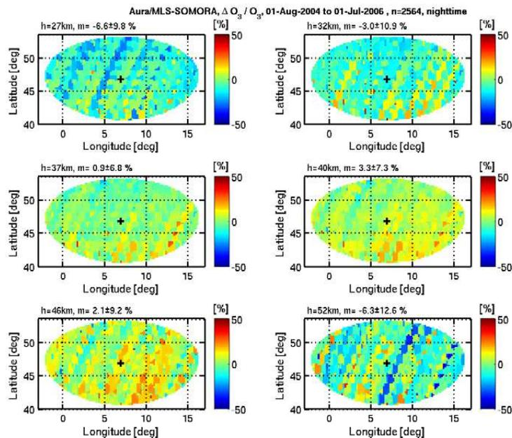
**Fig. 8.** Geographic map of nighttime ozone differences  $\Delta O_3 / \bar{O}_3$ . The location of the ground station is indicated by the cross (center of the map). Faint stripes along the satellite sub-orbital tracks are observed.
