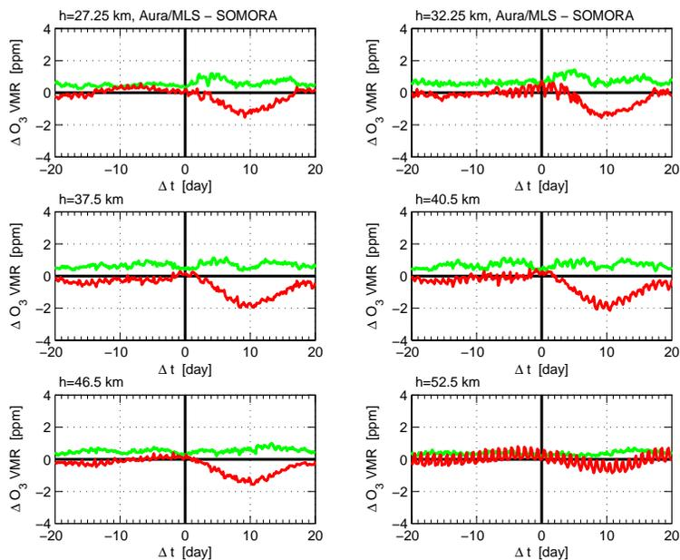
**Fig. 7.** Dependence of  $O_3$  differences (Aura/MLS – SOMORA) on the time lag  $\Delta t = t_{\text{SOMORA}} - t_{\text{Aura/MLS}}$ . Nighttime Aura/MLS measurements from 10 January to 20 January 2005 have been selected. The red line denotes the mean bias, and the green line is the standard deviation.
