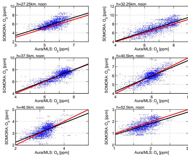
**Fig. 3.** Scatter plots of coincident O<sub>3</sub> VMR measurements of Aura/MLS and SOMORA at altitudes 27, 32, 37, 40, 46, and 52 km around noon. The black line is the best fit straight line, while the red line would be obtained for a perfect agreement ( $O_3(\text{SOMORA})=O_3(\text{Aura/MLS})$ ).
