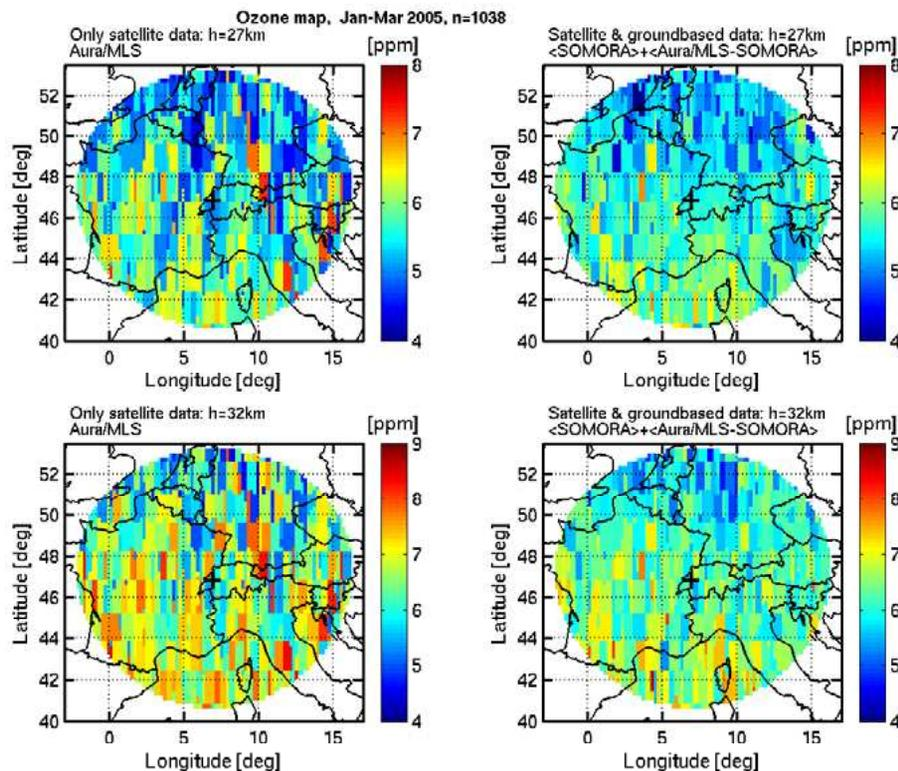
**Fig. 19.** Mean ozone maps around Payerne (black cross). The maps on the left-hand-side are calculated by using Aura/MLS profiles during January–March 2005. The temporal noise in the ozone maps is significantly reduced when the space-based measurements are combined with the ground-based measurements of the SOMORA radiometer in Payerne (ozone maps on the right-hand-side).
