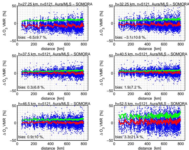
**Fig. 6.**  $O_3$  differences (blue dots) as function of the horizontal distance between the sounding volumes of Aura/MLS and SOMORA. The red line indicates the mean bias (moving average over 50 profile pairs) as function of the horizontal distance while the green line denotes the related standard deviation  $\sigma$ .
