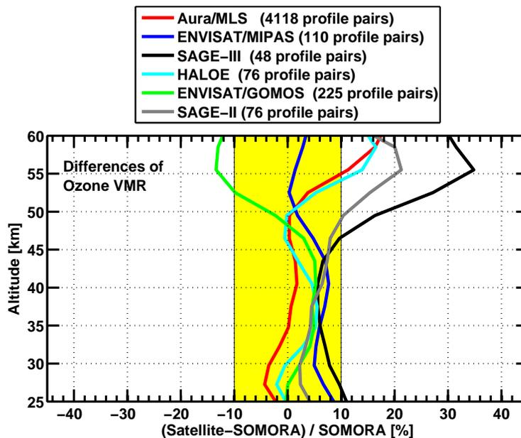
**Fig. 1.** Mean differences of the observed  $O_3$  volume mixing ratios of satellite limb sounders with respect to the ground station SOMORA in Payerne. Averaging kernel smoothing (Eq. 1) has been applied.
