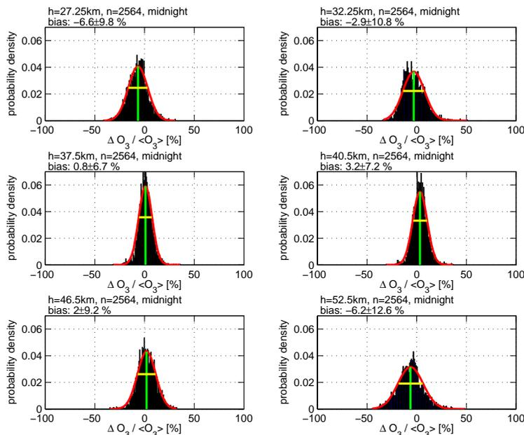
**Fig. 4.** Probability density function of the  $O_3$  vmr differences Aura/MLS – SOMORA ( $\Delta O_3 / \bar{O}_3$ ) around midnight. The numbers of profile pairs  $n$  and the altitudes are given at the top of the graphs. The red line is the fit of the Gaussian normal distribution to the data. The green line indicates the bias (mean average), and the yellow line denotes the range of  $2\sigma$ , where  $\sigma$  is the standard deviation.
