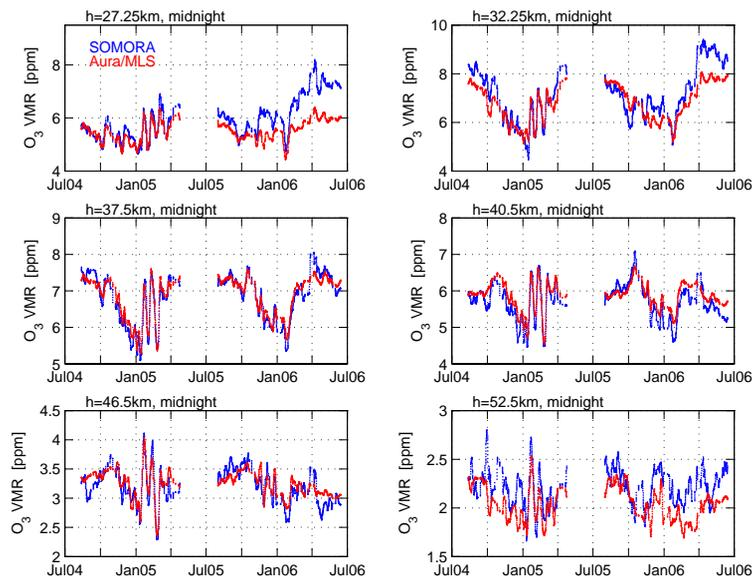
**Fig. 10.** Time series of nighttime  $O_3$  VMR of SOMORA (blue line) and Aura/MLS (red line). Averaging kernel smoothing has been applied to the series of the Aura/MLS measurements which are coincident with the SOMORA measurements. Short temporal fluctuations (periods  $<4$  days) are suppressed by a moving average over 30 data points of both time series.
