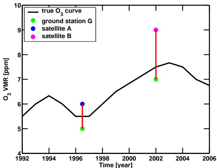
**Fig. 16.** Scheme of cross-validation by double differencing: Measurements of satellites *A* and *B*, separated in time, are compared by using the long-term data set of ground station *G* (the satellite measurements are nearby the ground station). The difference of lengths of the red lines is estimated to be the difference of the systematic errors of the satellites *A* and *B*. The black curve is the unknown time series of true ozone at a fixed altitude over the ground station.
