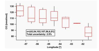
**Fig. 2.** Longitudinal profile of the CO median mixing ratio in the altitude range 0–1 km a.s.l.; red bar denotes the median; the lower and upper boundary of the red box mark the 25% and 75% percentiles, the bottom and top whisker the 10% and 90% percentiles.
