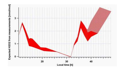
**Fig. 10.** Expected  $H_2O_2$  mixing ratios along the 57 different trajectories prescribed by the varying *k* values. The variation of the mixing ratio as a function of local time arises from the measured longitudinal gradient, the effect of the different starting times of the trajectories and the superimposed diurnal cycle.
