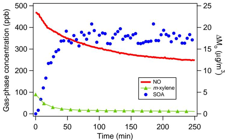
**Fig. 1.** Typical reaction profile of a high-NO<sub>x</sub> experiment in which HONO is used as the OH precursor (initial conditions: 89.3 ppb of *m*-xylene, 470 ppb NO, and 473 ppb NO<sub>2</sub>).
