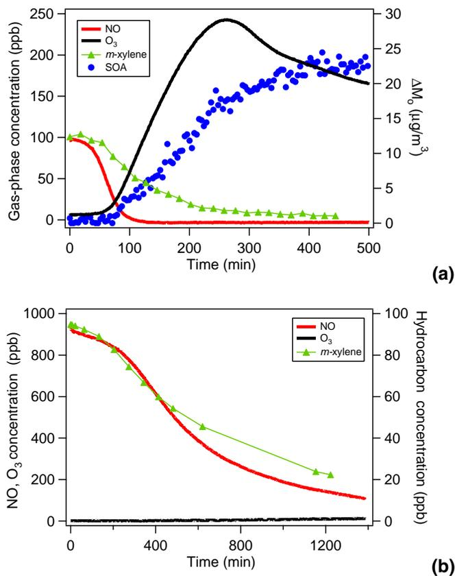
**Fig. 2.** (a) Reaction profile of a typical classical photooxidation experiment (initial conditions: 101.6 ppb *m*-xylene, 97 ppb NO, and 26 ppb  $\text{NO}_2$ ). (b) Reaction profile of a classical photooxidation experiment in the presence of  $\sim 1$  ppm  $\text{NO}_x$  (initial conditions: 94.8 ppb *m*-xylene, 878 ppb NO, and 65 ppb  $\text{NO}_2$ ). A negligible amount of ozone is formed during the experiment, and no SOA is formed.
