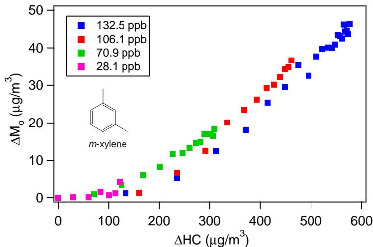
**Fig. 3.** Time-dependent growth curves for *m*-xylene photooxidation under high- $\text{NO}_x$  conditions. The concentrations in the legend refer to the amount of *m*-xylene reacted in each experiment.
