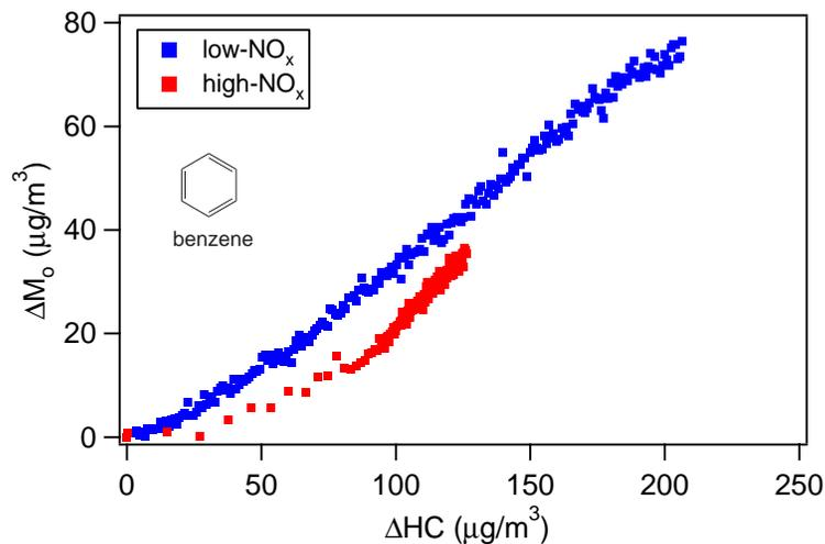
**Fig. 5.** Time-dependent growth curves for benzene photooxidation under high- and low- $\text{NO}_x$  conditions. Under high- $\text{NO}_x$  conditions, the initial benzene concentration is 337 ppb (12% reacted). Under low- $\text{NO}_x$  conditions, the initial benzene concentration is 395 ppb (16% reacted) and the system has a constant yield of 37%.
