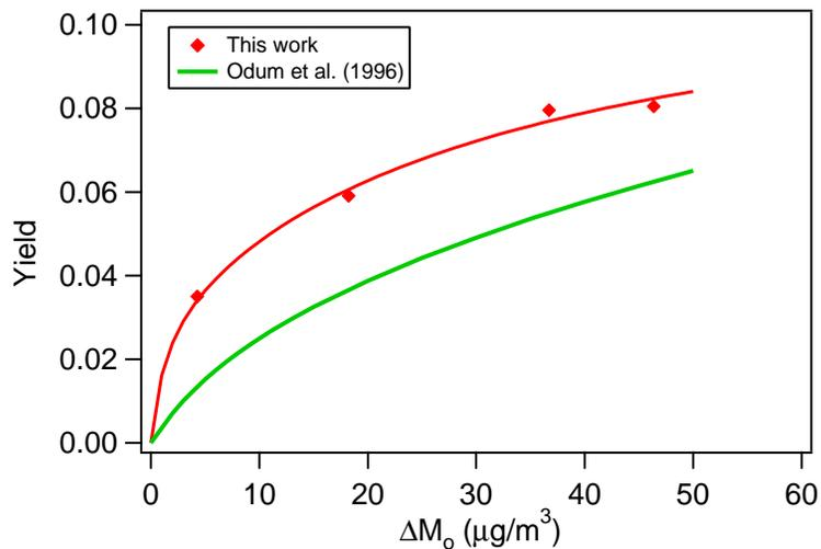
**Fig. 11.** Comparison of *m*-xylene high-NO<sub>x</sub> yield curve obtained in the current work to that from Odum et al. (1996). The yield curve from Odum et al. (1996) has been corrected for the temperature (25°C) of this study and density (1.48 g cm<sup>-3</sup>) of the SOA.
