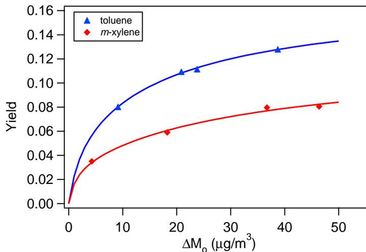
**Fig. 8.** Yield curves for toluene and *m*-xylene under high-NO<sub>x</sub> conditions. The parameters for fitting the yield curves are, toluene:  $\alpha_1 = 0.058$ ,  $K_{om,1} = 0.430$ ,  $\alpha_2 = 0.113$ , and  $K_{om,2} = 0.047$ ; *m*-xylene:  $\alpha_1 = 0.031$ ,  $K_{om,1} = 0.761$ ,  $\alpha_2 = 0.090$ , and  $K_{om,2} = 0.029$ .
