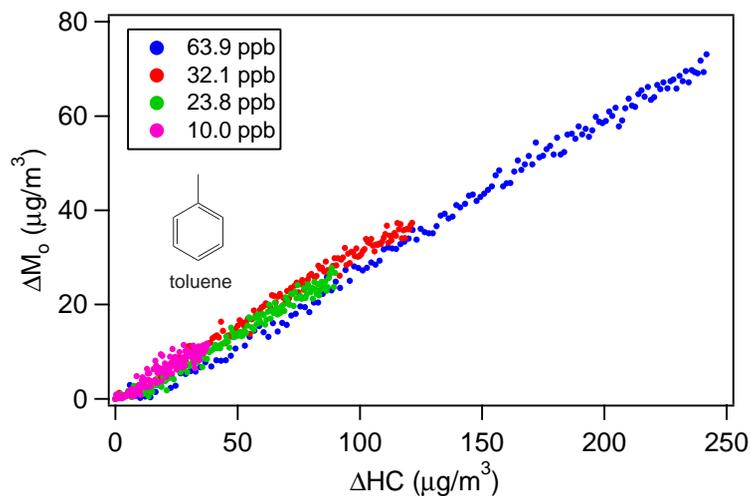
**Fig. 7.** Time-dependent growth curves for toluene photooxidation under low- $\text{NO}_x$  conditions. The concentrations in the legend refer to the amount of toluene reacted in each experiment. The system exhibits a constant yield of 30%.
