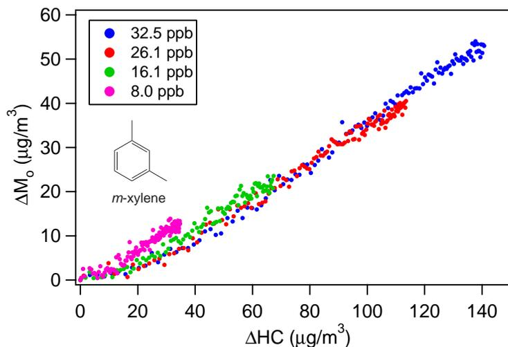
**Fig. 6.** Time-dependent growth curves for *m*-xylene photooxidation under low- $\text{NO}_x$  conditions. The concentrations in the legend refer to the amount of *m*-xylene reacted in each experiment. The system exhibits a constant yield of 36%.
