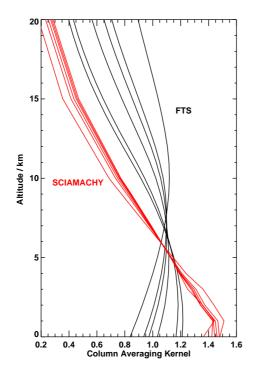
**Fig. 2.** Example averaging kernels, for various solar zenith angles (i.e. air masses), for SCIA-MACHY (red line) and the FTS (black line) highlighting the different sensitivity of each instrument to the lower troposphere. The SCIAMACHY averaging kernels are calculated numerically (see, e.g. Barkley et al., 2006c).
