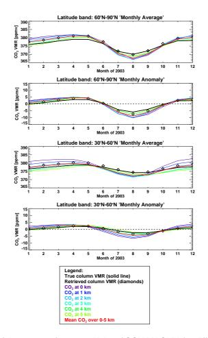
**Fig. 3.** Assessment of the near surface sensitivity of SCIAMACHY, for different latitude regions, using the 2003  $CO_2$  climatology. The plots show the the retrieved and true column VMRs against  $CO_2$  mixing ratios within the lower troposphere both in terms of absolute magnitudes and also the anomalies.
