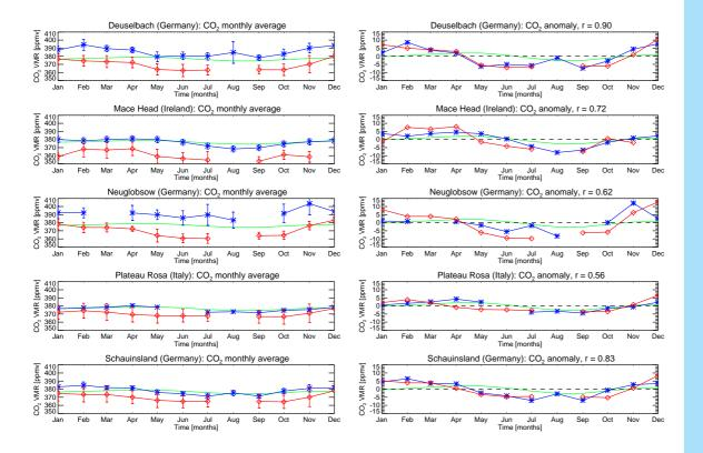
**Fig. 9.** Time series of ground based European in situ observations (blue) versus SCIAMACHY  $CO_2$  (red). The  $1\sigma$  error bars are shown on the monthly averages. The a priori  $CO_2$  column VMR is shown in green.
