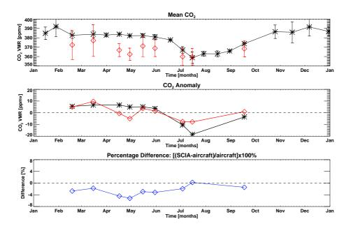
**Fig. 5.** The  $CO_2$  time series over Yakutsk for SCIAMACHY (red) and aircraft (black). Top panel: The mean aircraft  $CO_2$  mixing ratio (over all altitudes) and the SCIAMACHY VMRs. The error bars represent the  $1\sigma$  uncertainty. Second panel: The  $CO_2$  anomaly (using only coincidental observations). Third panel: The percentage difference between SCIAMACHY and the mean aircraft  $CO_2$  mixing ratio (over all altitudes).
