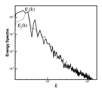
**Fig. 4.** Inertial range velocity spectra showing  $\mathcal{E}_x(k)$  and  $\mathcal{E}_y(k)$  components of energies in the compressible fluctuations. Notice the spectral disparity at the lower *k*-modes. This indicates that larger scales show a greater propensity for anisotropization. The two spectra are isotropic for larger *k* (i.e.  $k \ge 50$ ).
