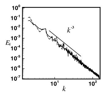
**Fig. 3.** Density (dashed curve) power spectrum from a decaying NI hydrodynamics simulation. The incompressible velocity fluctuations (solid curve) follow a Kolmogorov spectrum close to  $\sim k^{-3}$  in a forward (or enstrophy) cascade regime of decaying turbulence. It is clear that density fluctuations are passively convected by the incompressible velocity fluctuations and exhibit nearly the same spectrum.
