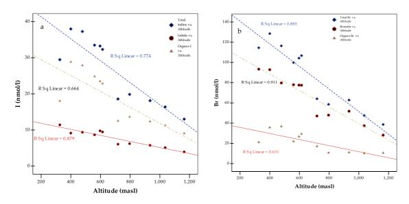
**Fig. 2. (a)** Total iodine, iodide and organically bound iodine in snow vs. altitude. **(b)** Total bromine, bromide, and organically bound Br in snow vs. altitude.
