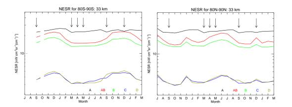
**Fig. 4.** Time series of NESR at 33 km tangent altitude for the 5 different spectral bands (A: 685–970 cm<sup>-1</sup>, AB: 1020–1170 cm<sup>-1</sup>, B: 1215–1500 cm<sup>-1</sup>, C: 1570–1750 cm<sup>-1</sup>, D: 1820–2410 cm<sup>-1</sup>). Southern Hemisphere gaps correspond to the missing Antarctic L2 profiles for July–August 2002 and October 2002. Arrows indicate decontamination events.
