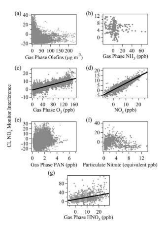
**Fig. 2.** Linear regression plots for the CL  $NO_x$  monitor interference plotted versus **(a)** gas phase olefins (CENICA), **(b)** gas phase  $NH_3$  (Santa Ana), **(c)** gas phase  $O_3$  (Pedregal), **(d)**  $NO_z$  (Pedregal), **(e)** gas phase PAN (CENICA), **(f)** particulate nitrate (La Merced), and **(g)** gas phase  $HNO_3$  (La Merced). See text for description of measurements. Results of the linear regressions are listed in Table 1.
