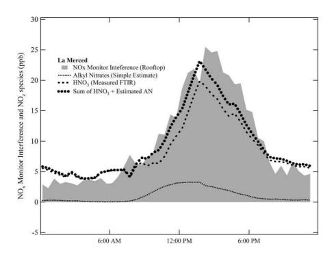
**Fig. 4.** Diurnally averaged profiles for measured CL  $NO_x$  monitor interference, measured  $HNO_3$  concentrations and calculated alkyl nitrate concentrations at La Merced site. Also included is a profile of the sum of the measured  $HNO_3$  concentration plus the estimated alkyl nitrate concentration (see text). Time of day is for local time.
