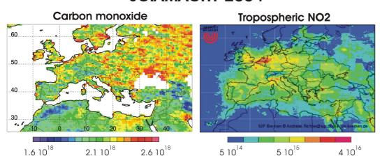
**Fig. 7.** Comparison of SCIAMACHY CO (left) and NO<sub>2</sub> (right) measurements over Europe for 2004 (the NO<sub>2</sub> has been retrieved at the University of Bremen by A. Richter Richter et al., 2005).
