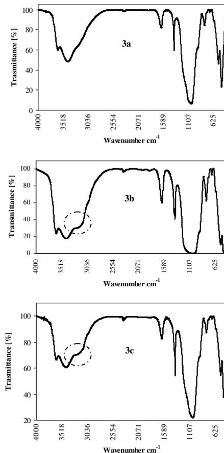
**Fig. 3.** The Fourier transform infrared (FT-IR) spectra of pure montmorillonite Fig. 3a, ammonia exposed montmorillonite Fig. 3b, degassed (after ammonia exposure) montmorillonite Fig. 3c with Bruker FTIR instruments, Model Vector 22. The absorption band at  $3220\text{ cm}^{-1}$  suggests chemi-adsorbed ammonia indicated by the dashed circle in Figs. 3b and 3c.
