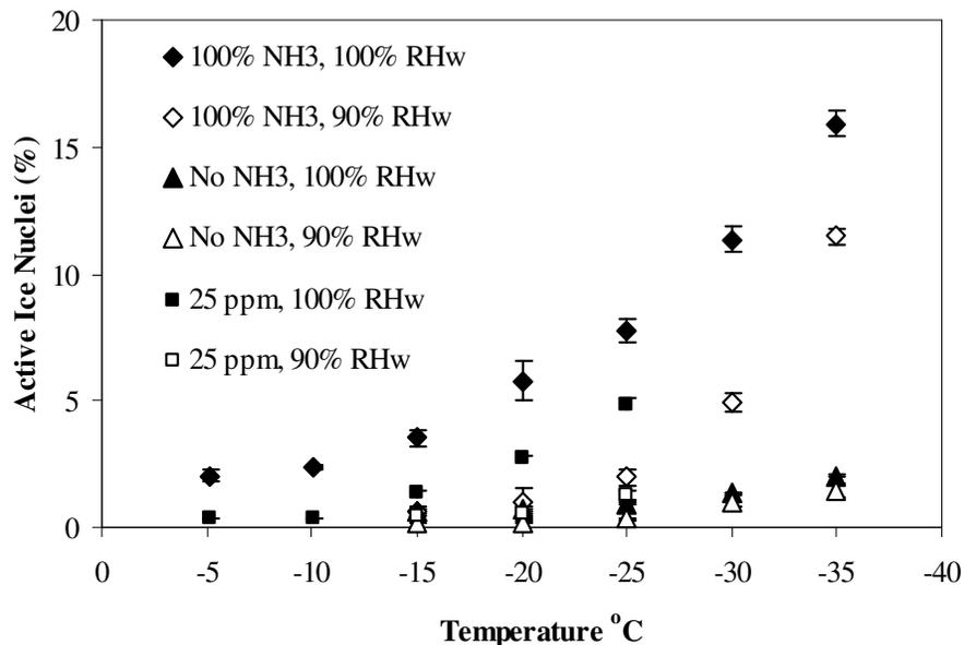
**Fig. 5.** Percentage of activated ice nuclei (as defined in Fig. 4) versus temperature (°C) of montmorillonite mineral dust particle exposed to 100% pure or 25 ppm ammonia gas and without ammonia gas exposure at 90% and 100% relative humidity with respect to water (RH<sub>w</sub>). The exposure time was 2 h for 100% pure ammonia and 18 h for 25 ppm ammonia. The vertical bars are the error bars equal to the standard deviation of the 15 measurements conducted at each temperature.
