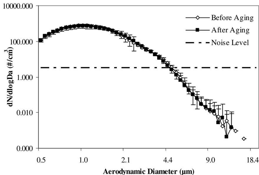
**Fig. 2.** Aerosol particle size distributions of montmorillonite mineral dust before and after aging with ammonia gas as measured with an Aerodynamic Particle Sizer (TSI 3321) exiting the aerosol generation of the CFDC. The dashed line indicates the noise level of the measurements determined by blank and dry experiments. The vertical bars are the error bars equal to the standard deviation of the 20 samples (duration of each sample is 60 s).
