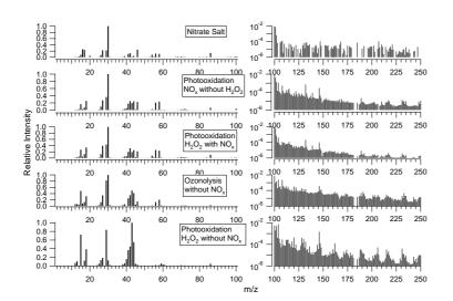
**Fig. 14.** cToF-AMS spectra (normalized to the largest peak) of aerosol generated from TEA oxidation under various conditions. In all cases, except for hydrogen peroxide without NO<sub>x</sub>, the nitrate salt was intentionally formed by mixing TEA with nitric acid in the chamber before the start of oxidation. All spectra were collected after the peak of aerosol growth had been reached.
