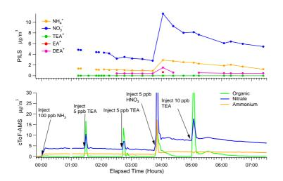
**Fig. 3.** Time series from exp. 19 in Table 2 of the cToF-AMS (bottom) and the PILS-IC (top) showing rapid particle growth and evaporation after TEA and nitric acid were added in small aliquots to a chamber containing equilibrated ammonium nitrate particles. The transient spikes in particle loading do not appear in the PILS-IC data because of the relatively long averaging time (5 min) of measurements and because the PILS-IC inlet is not in the path of the highly concentrated injection plume.
