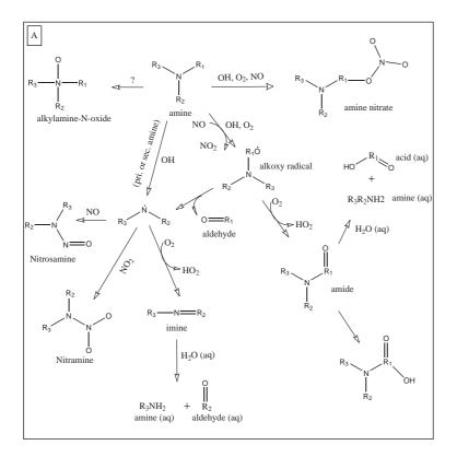
**Fig. 5.** Mechanisms of amine oxidation by: **(A)** OH in the presence of  $NO_x$  (Schade and Crutzen, 1995), **(B)** Ozone, in the absence of  $NO_x$  (Tuazon et al., 1994), **(C)** OH in the absence of  $NO_x$ .
