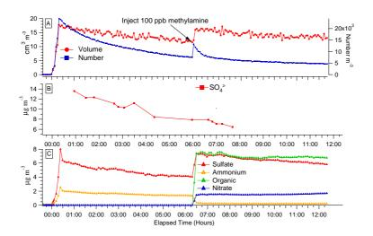
**Fig. 4.** Time Series of data from the DMA Panel (**A**), PILS-IC Panel (**B**), and cToF-AMS Panel (**C**) showing rapid replacement of ammonium sulfate by methylammonium sulfate during the injection of 100 ppb of methylamine into a chamber containing ammonium sulfate seed and ozone. The increase in the ratio of organic signal to sulfate signal near the end of the experiment results from the slow reaction of methylamine with ozone forming a small mass of organic aerosol.
