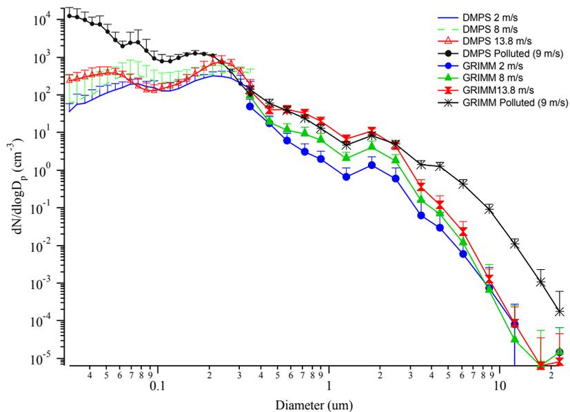
**Fig. 4.** Comparison of the number size distributions at different wind speeds for clean marine air and a polluted episode. The upper end of the DMPS spectra at the overlap with the GRIMM OPC are not shown for clarity, neither are the negative error bars. Errors shown are 1 standard deviation.
