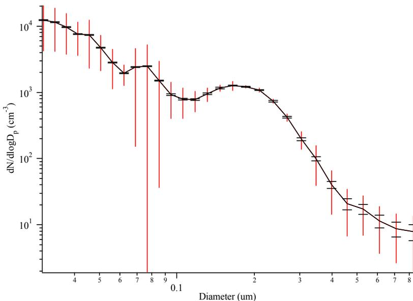
**Fig. 6.** Comparison of the different errors associated with the DMPS data. The vertical lines are the standard deviation over 1 h (26 October 2003 18:00–19:00) and the bars are the errors based on Poisson statistics averaged over the same hour.
