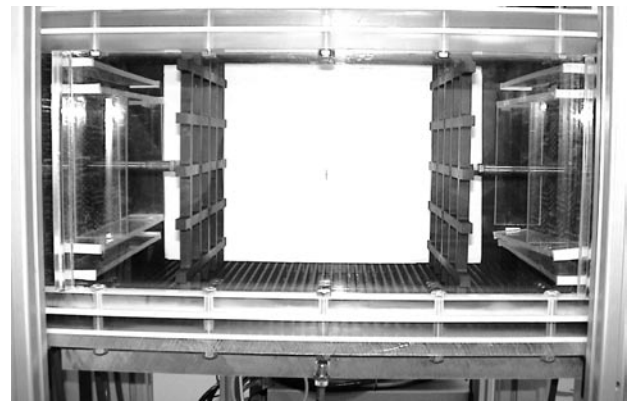
Fig. 2. The test section of the oscillating grids turbulence generator.
