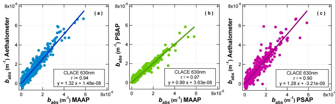
**Fig. 2.** Comparison of the absorption coefficients measured by the MAAP, the Aethalometer, and the PSAP downstream of the total inlet. Symbols represent 1-h averages (total 1626 h).
