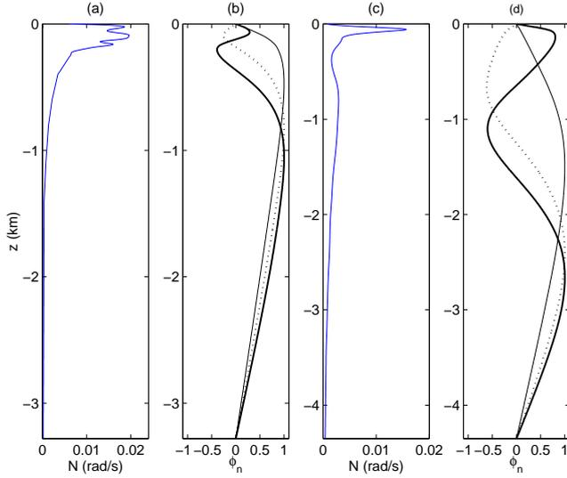
**Fig. 1.** The profiles of  $N$  for the Sulu Sea (a), and the Bay of Biscay (c), after Apel et al. (1985) and Pingree and New (1991), respectively. The corresponding modal structures ((b) and (d)) have been obtained by solving Eq. (3); the first, second and third modes are indicated by thin, dotted and thick lines, respectively.
