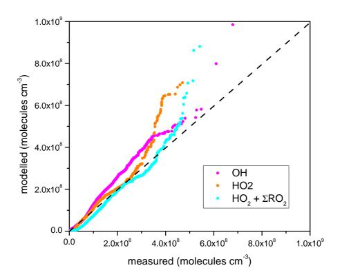
**Fig. 9.** QQ plot showing simultaneous modelled and measured OH (pink),  $HO_2$  (orange) and  $(HO_2 + \Sigma RO_2)$  (blue) concentrations. OH data are multiplied by 100,  $HO_2$  by two and  $(HO_2 + \Sigma RO_2)$  is divided by 3. A 1-1 line is shown for comparison.
