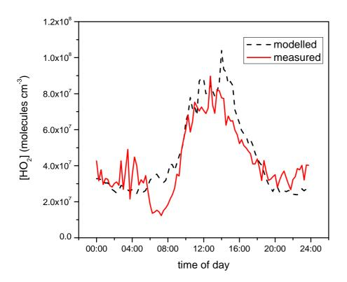
**Fig. 4.** 15-min average modelled and measured  $HO_2$  concentrations plotted as a diurnal time series. Modelled data are in grey, measured data are black. (Number of data points contributing to the mean measured data varies between 23 and 96).
