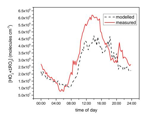
**Fig. 7.** 15-min average modelled and measured  $[HO_2 + \Sigma RO_2]$  concentrations plotted as a diurnal time series. Modelled data are black dashed lines, measured data are red. (Number of data points contributing to the mean measured data varies between 22 and 96).
