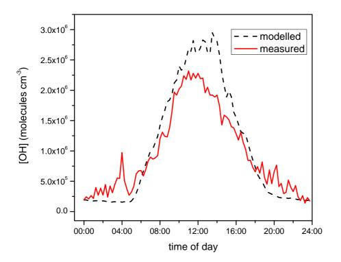
**Fig. 2.** 15-min average modelled and measured OH concentrations plotted as a diurnal time series. Modelled data are dashed black lines, measured data are red. (Number of data points contributing to the mean measured data varies between 20 and 85).
