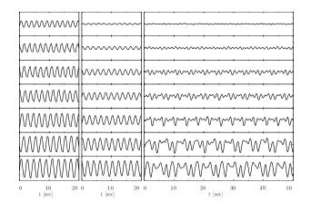
**Fig. 7.** Temperature close to the inner wall of the modulated cylindrical annulus as recorded by thermistors at the positions y = -6.1, -0.8 and +0.6 (from left to right) in the case  $\eta = 458, \delta = 0.45, P = 0.71$ . The Rayleigh numbers (calculated without consideration of the convective contribution to the heat transport) are 9003, 10033, 11007, 12012, 12915, 13795 (from top to bottom).
