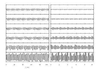
**Fig. 8.** Comparison of time dependences of temperatures measured by a thermistor at the position y = 4.7 with temperature dependences at the same y-position (x = -0.4) obtained from numerical simulations in the case  $\eta = 458$ ,  $\delta = 0.45$ ,  $\alpha_M = 0.296$ . The Rayleigh numbers used in the simulations are 2385, 3500, 3600, 3900, 4000, 4250, 4500 (from top to bottom).
