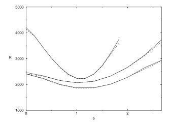
**Fig. 2.** Critical Rayleigh number  $R_c$  for onset of convection as a function of  $\delta$  in the cases  $\eta = 600$  with  $\alpha_M = 1.0$ ,  $\eta = 300$  with  $\alpha_M = 1.0$  and with  $\alpha_M = 0.5$  (from top to bottom). For each of the three cases the results for vanishing Floquet wavenumber, d = 0 (solid curves) and for finite values of *d* (dashed curves) are shown. P = 0.71 in all cases.
