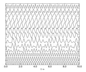
**Fig. 6.** Time dependence of the temperature  $\Theta(x, y, t)$  at x = -0.4 and at the values  $y = 2 \cdot m$  with m = 0, 1, ..., 12 (from bottom to top) in the case R = 4000,  $\eta = 300$ ,  $\alpha_M = 0.25$ ,  $\delta = 0.4$ , P = 0.71.
