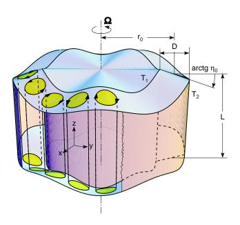
Fig. 1. Geometrical configuration of the rotating modulated cylindrical annulus.
