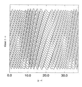
**Fig. 5.** The temperature  $\Theta$  at the point x = -0.4 as a function of *y* at different instances in time,  $t = t_0 + n\Delta t$ , *n* increasing from bottom to top with  $\Delta t = 0.06$ , in the case R = 3000,  $\eta = 300$ ,  $\alpha_M = 0.25$ ,  $\delta = 0.3$ , P = 0.71.
