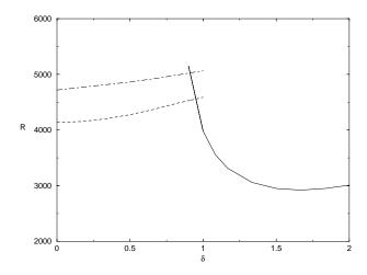
**Fig. 3.** Critical Rayleigh number  $R_c$  for onset of convection as a function of  $\delta$  in the case  $\eta = 600$  with  $\alpha_M = 3.0$  and P = 0.71. The dotted (dash-dotted) curve corresponds to the onset of thermal Rossby waves with finite (vanishing) value of d. The solid curve corresponds to the steady pinned mode of convection.
