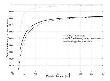
**Fig. 1.** Transport efficiency of a TSI3025 CPC and the heating tube (at 280°C) used in the V-SMPS setup as a function of particle size. The detection efficiency of the CPC (dotted line) is taken into account in the inversion of the data; the penetration efficiency of the heating tube (solid line) is considered in the final size distribution correction.
