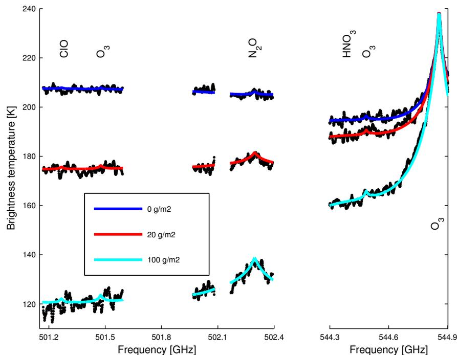
**Fig. 1.** Simulated and measured spectra of the Odin-SMR stratospheric mode. Tangent altitude is 7 km. Solid (coloured) lines are simulated spectra for different cloud ice columns. The assumed cloud layer extends between 12 and 15 km, with the ice vertically equally distributed. Dots (black) represent examples on measured spectra (at 10 MHz resolution, compared to the nominal value of 2 MHz).
