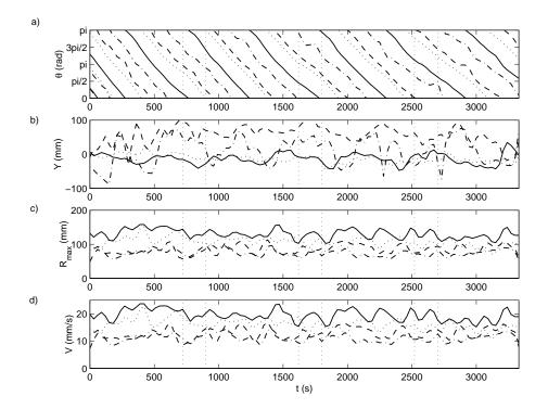
Fig. 5. Time series of the vortex characteristics: (a) Spatial phase of the vortex centres; (b) lateral distance of the vortex centre from the disk edge; (c) major radius of the vortices; and (d) maximum circulation velocity in the vortex. The solid line is for the primary anticyclone, the dotted line for the primary cyclone, the dashed line for the secondary anticyclone, and the dash-dotted line for the secondary cyclone.
