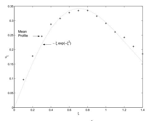
**Fig. 4.** Typical mean velocity profile. Superimposed is the function  $0.8\xi \exp(-\xi^2)$ .
