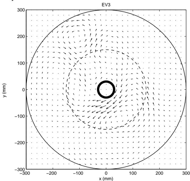
**Fig. 13.** Third EOF from the EOF analysis of the set of rotated eddy fields.
