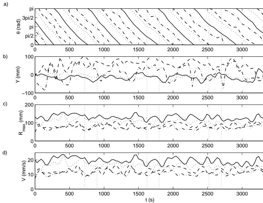
**Fig. 5.** Time series of the vortex characteristics: **(a)** Spatial phase of the vortex centres; **(b)** lateral distance of the vortex centre from the disk edge; **(c)** major radius of the vortices; and **(d)** maximum circulation velocity in the vortex. The solid line is for the primary anticyclone, the dotted line for the primary cyclone, the dashed line for the secondary anticyclone, and the dash-dotted line for the secondary cyclone.
