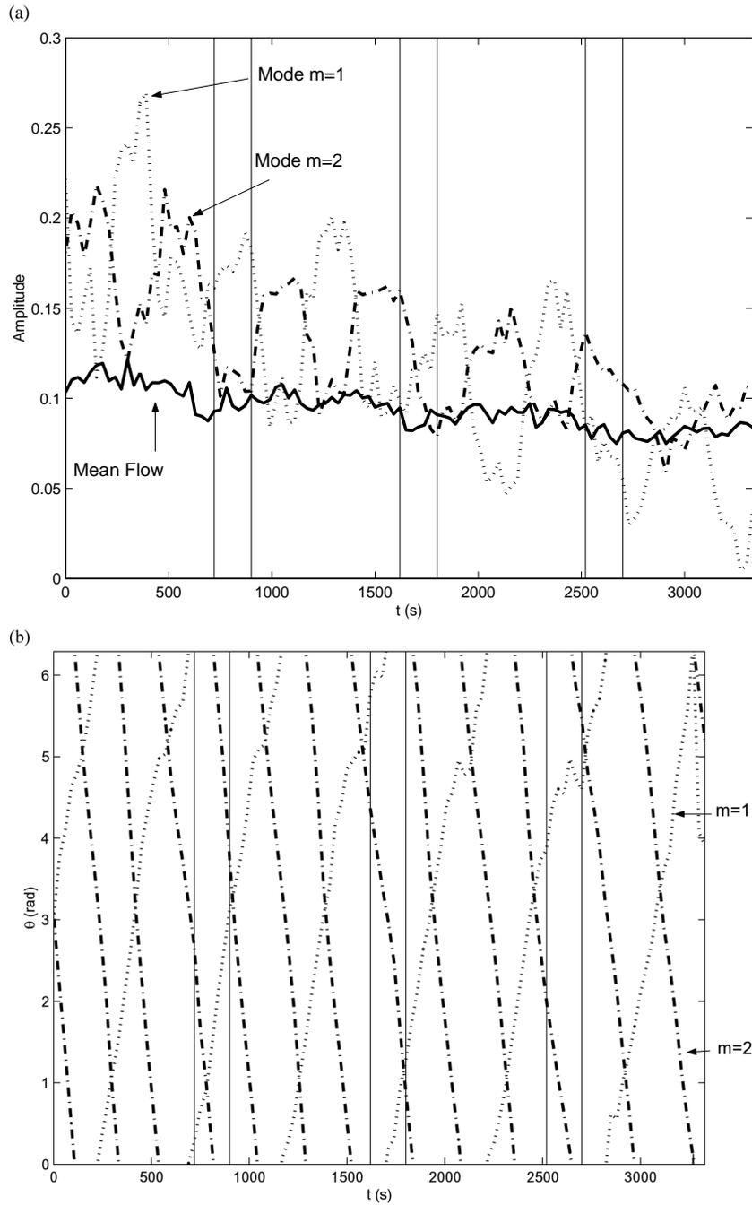
**Fig. 9.** Time series of the Principal Components from the EOF analysis of the set of full field data. All PCs are scaled with their singular value. **(a)** Amplitude of the first principal component (solid line) and “mode amplitudes” of the two successive pairs of principal components,  $PC_2$  and  $PC_3$  as the dash-dotted line, and  $PC_4$  and  $PC_5$  as the dotted line. **(b)** Phase of the pair  $PC_2$  and  $PC_3$  (dash-dotted line) and  $PC_4$  and  $PC_5$  (dotted line).
