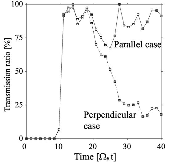
**Fig. 9.** Pump wave energy detected at the end of the simulation box ( $X\Omega_e/C_v = 10.24$ ) as a function of time. Up to  $\Omega_e t = 20$ , the two profiles are approximately the same. But in the perpendicular case, the coupling process can continue since the ECH waves propagation characteristics are not very sensitive to the plasma temperature. The transmission of the pump wave is therefore much reduced.
