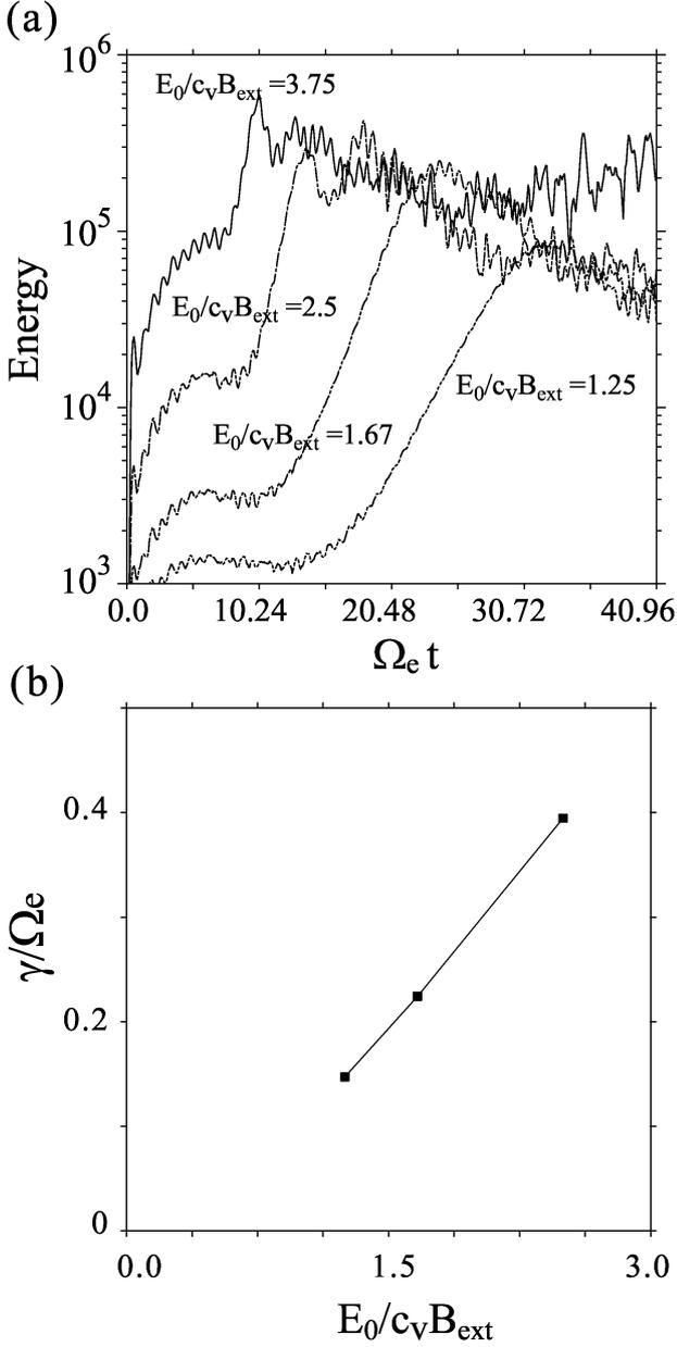
**Fig. 5.** Relationship between the starting time of the three-wave coupling process and the amplitude of the pump wave. Panel (a) shows the time evolutions of the energy of ES waves excited in the three-wave coupling process with different amplitudes of the pump wave. Panel (b) shows the temporal growth rates for  $E_0/|B_{ext}C_v| = 1.25, 1.67,$  and  $2.5$  obtained from the slope of data in panel (a) in a time interval where the wave energy grows exponentially.
