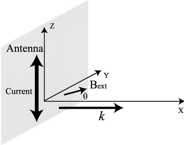
**Fig. 2.** Geometry of the simulation experiment in the 1-D case. The pump wave is emitted at the origin of the system by a current  $J_z$  injected by an antenna. The angle between  $\mathbf{B}_{ext}$  and the propagation vector can be changed.
