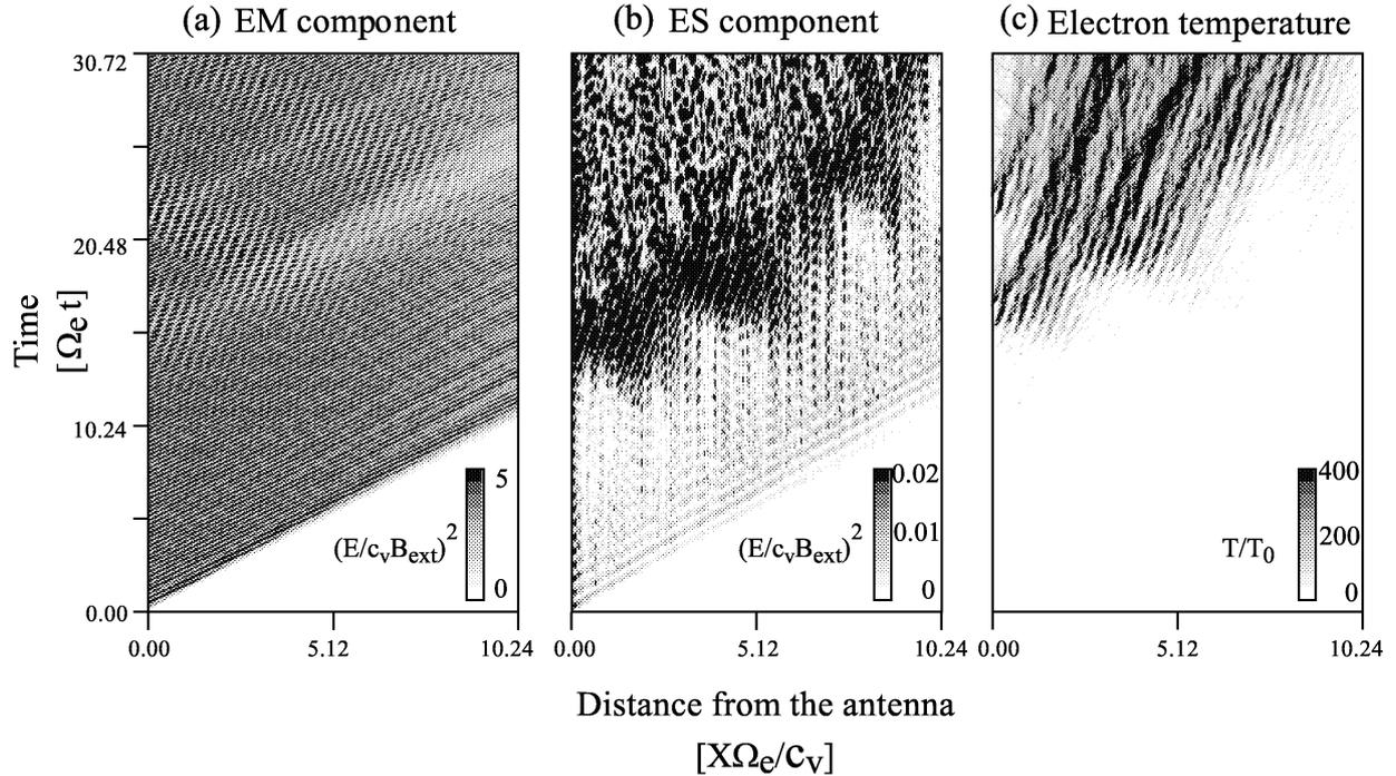
**Fig. 4.** Evolution of the wave field and of the electron temperature as a function of time and distance. From left to right: EM pump wave energy ( $E_z$ ), excited ES wave energy ( $E_x$ ), electron temperature ( $T_e$ ). In this simulation run, the pump wave intensity  $E_0/|\mathbf{B}_{ext}C_v|$  is equal to 2.5.
