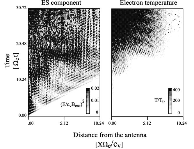
**Fig. 8.** Excited ES component and associated electron temperature for a case where  $\mathbf{B}_{ext}$  is along the  $y$  direction which is perpendicular to both directions of the pump wave propagation and current oscillation of antenna. The intensity of the pump wave is constant and equal to  $E_0/|\mathbf{B}_{ext}C_v| = 2.5$ .
