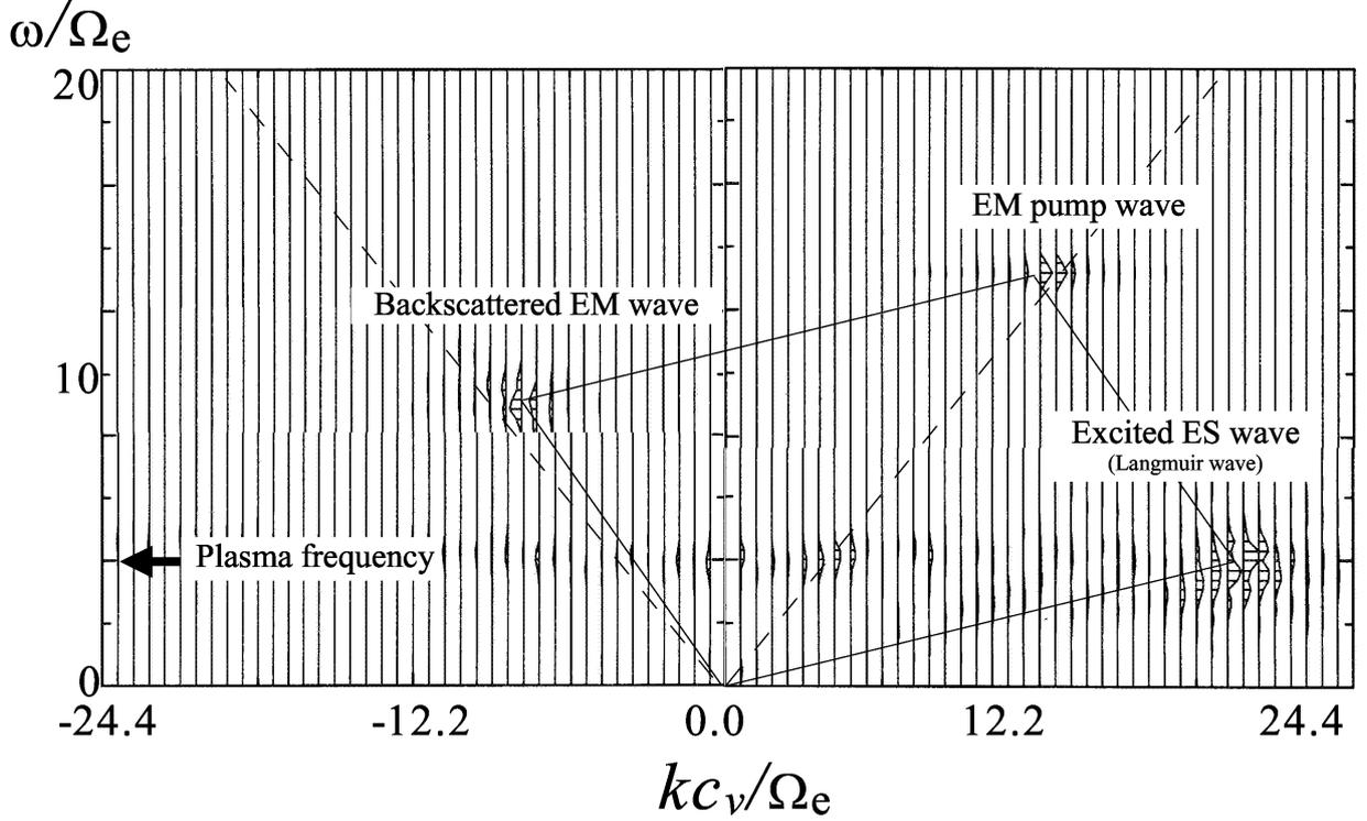
**Fig. 3.**  $\omega - k$  diagram obtained by the Fourier transformation of  $E_z$  electromagnetic and  $E_x$  electrostatic data in space and time for the parallel case. The obtained wave spectra are plotted at each wavenumber, normalized to their maximum value. The dashed lines correspond to the speed of light. The wavenumber of the most intense electrostatic wave corresponds approximately to  $kC_v/\Omega_e \sim 20$ .
