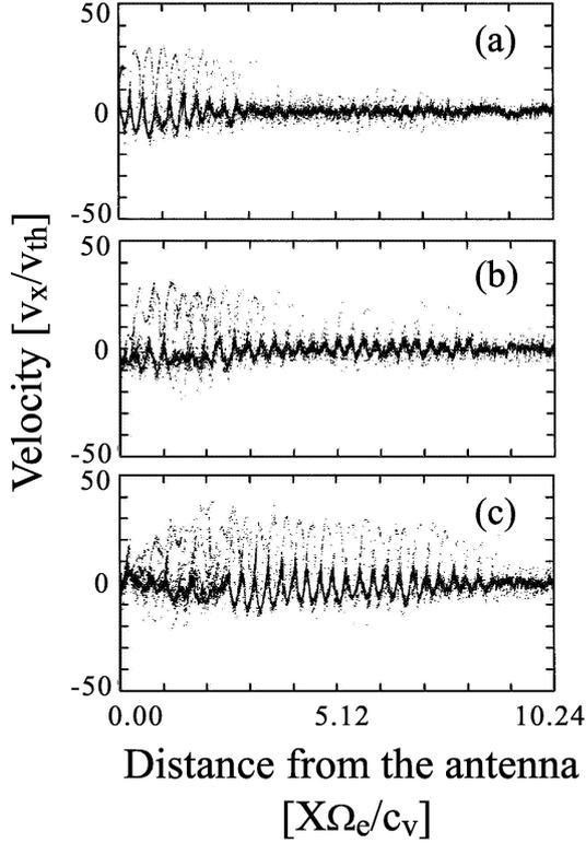
**Fig. 7.** Phase diagrams of electrons in a plane of  $V_x$  versus  $x$  at different times: (a)  $\Omega_e t = 14.08$  (b) 16.64, and (c) 19.20. The velocity values are normalized to the initial thermal velocity of electrons.
